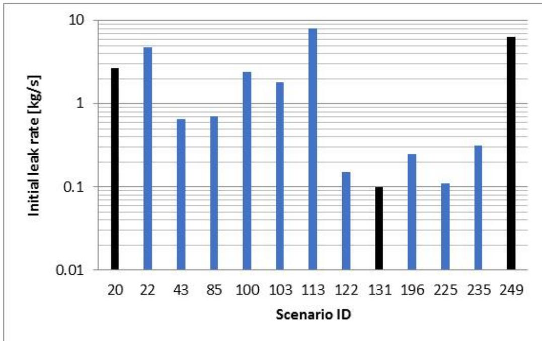
Figure 3.25 – Initial leak rate for hose leaks on NCS 2001 – 2017. The y-axis is in logarithmic scale
