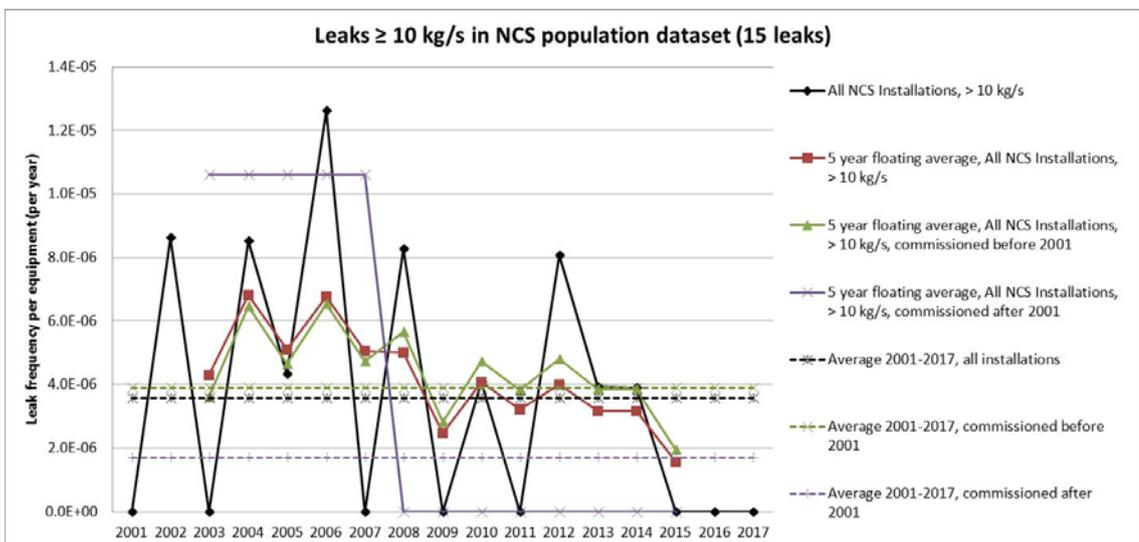
Figure 5.6 - Average frequency and floating average for leaks ( $\geq 10$  kg/s) per component versus time. Floating average plotted versus the middle year of the period that is averaged (*i.e.* the data point for year 2012 applies for the period 2010-2014)
