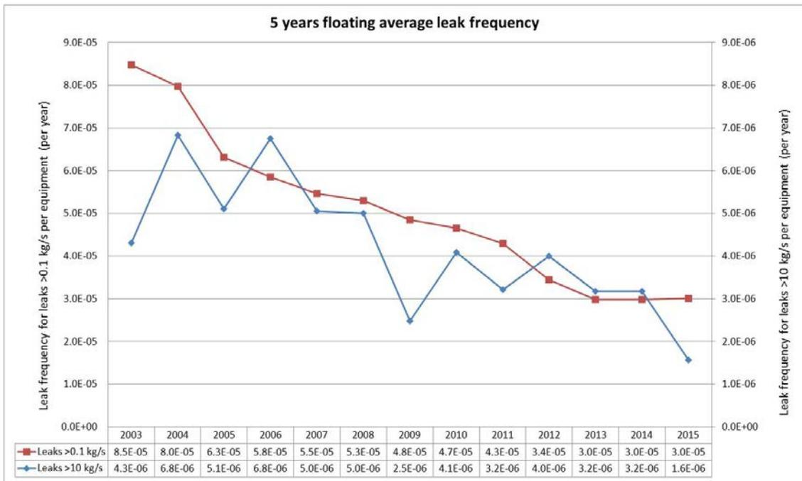
Figure 5.7 – 5 years floating average frequency for leaks  $\geq 0.1$  kg/s and  $\geq 10$  kg/s per equipment for various time periods. Floating average plotted versus the middle year of the period that is averaged (*i.e.* the data point for year 2012 applies for the period 2010-2014). Note that the blue curve relates to the right axis
