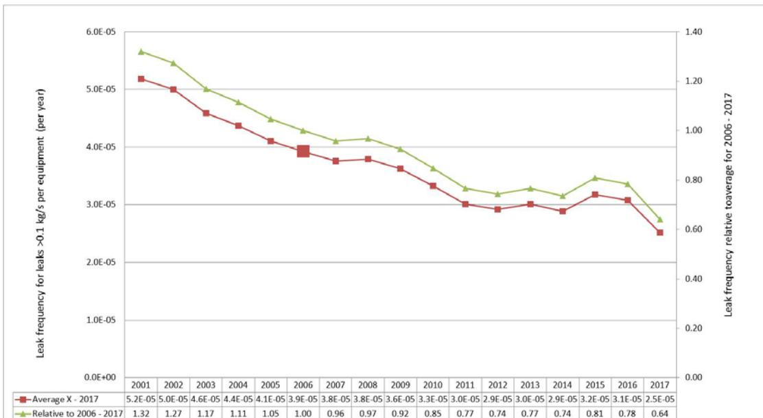
Figure 5.8 – Average leak frequency from year x to 2017 (red curve). The x- value is the value on the x-axis. The average for 2006 – 2017 is marked with a large marker. The green curve shows the average leak frequency for year x – 2017 relative to the average leak frequency for 2006 – 2017 (right y-axis)
