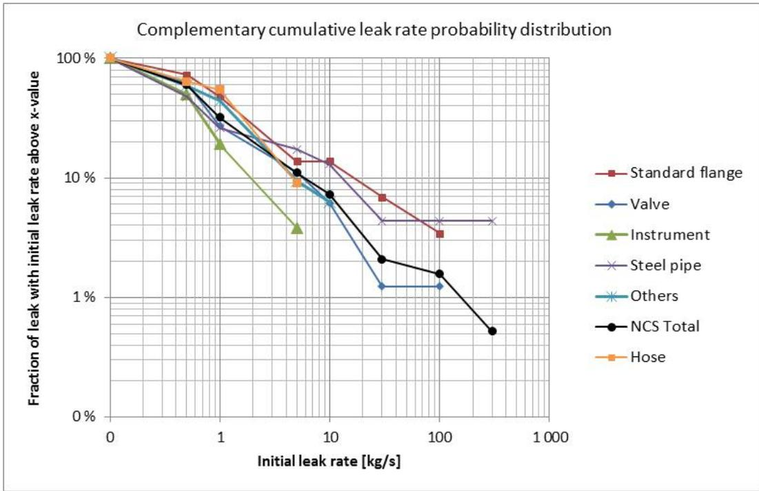
Figure 3.15 - Complementary cumulative probability distribution with respect to initial leak rate for Significant NCS leaks, including Hose leaks. Note that the leaks are categorized into leak rate categories. See also text above
