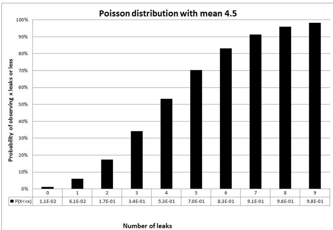
Figure 6.3 – Probability of observing x number of leaks or less with leak rate >10 kg/s, given expected number of leaks is 4.5
