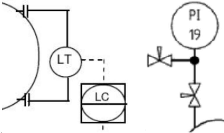
Figure 3.6 - Examples instrument connections
