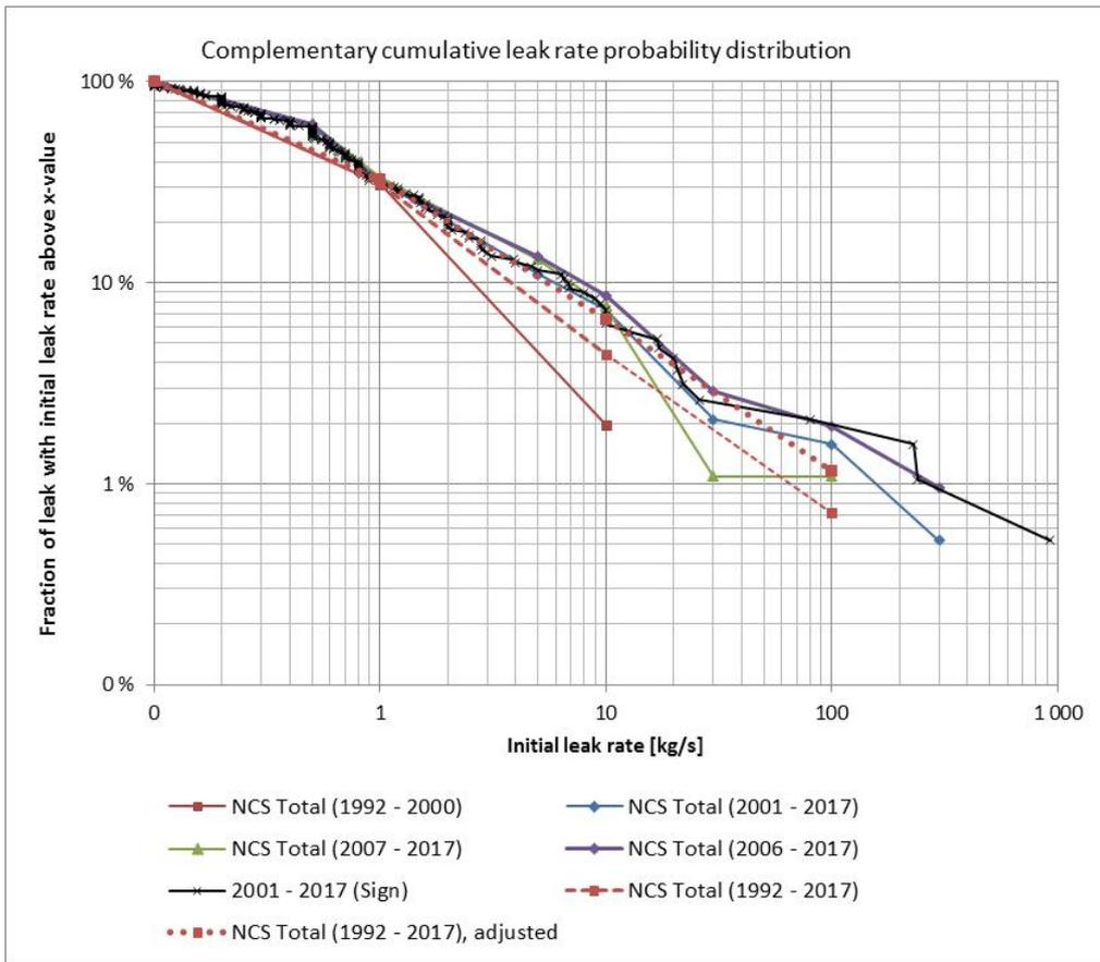
Figure 3.20 - Complementary cumulative probability distribution with respect to initial leak rate for Significant NCS leaks (total leaked quantity >10 kg, see TN-4) for different data periods
