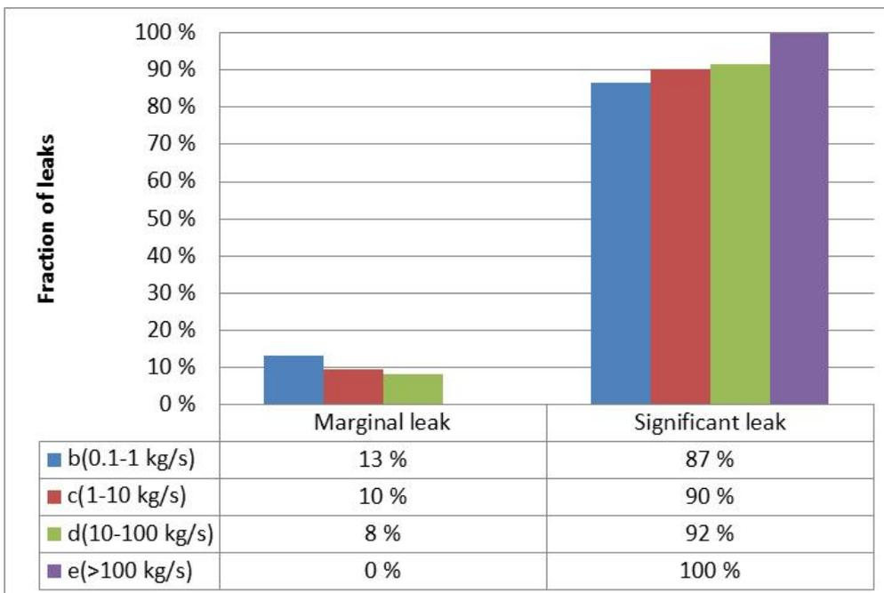
Figure 3.2 - Relative distribution of all NCS leaks (217) per leak scenario. The contributions from Marginal and Significant leaks sum up to 100%
