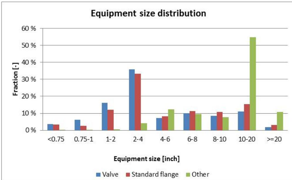
Figure 4.14 – Equipment size distribution for valve, standard flange and other equipment. Other equipment excludes hose and instrument (and valve and standard flange) as they are all ½" or ¾". All 90 installations being in operation in the period 2001 – 2017 are included
