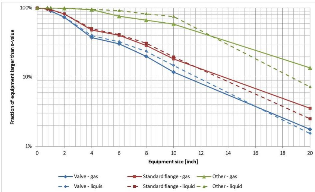
Figure 4.13 – Fraction of equipment that have a larger dimension than specified on the x-axis. Equipment containing gas and liquid separately. All 90 installations being in operation in the period 2001 – 2017 are included. Other equipment excludes hose and instrument (and valve and standard flange) as they are all 3/4"
