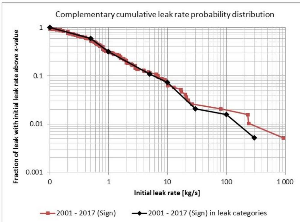
Figure 3.13 - Complementary cumulative probability distribution with respect to initial leak rate for Significant leaks (total leaked quantity >10 kg, see TN-4), based on logged leak rate and grouped in categories
