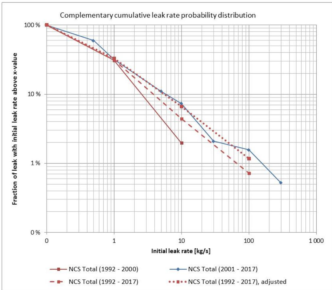
Figure 3.19 - Complementary cumulative probability distribution with respect to initial leak rate for Significant NCS leaks (total leaked quantity >10 kg, see TN-4) in period 2001 – 2017, together with corresponding curves including data from the period 1992-2000
