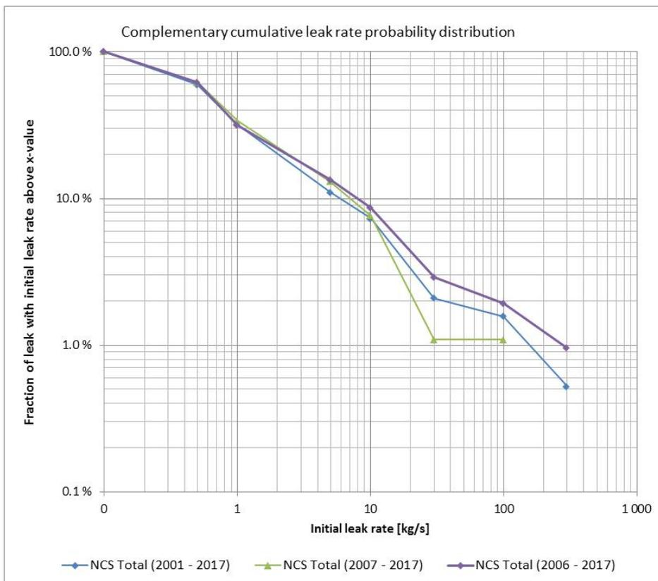
Figure 3.17 - Complementary cumulative probability distribution with respect to initial leak rate for Significant NCS leaks (total leaked quantity >10 kg, see TN-4) for different data periods. Note that the leaks are categorized into leak rate categories. See also text above
