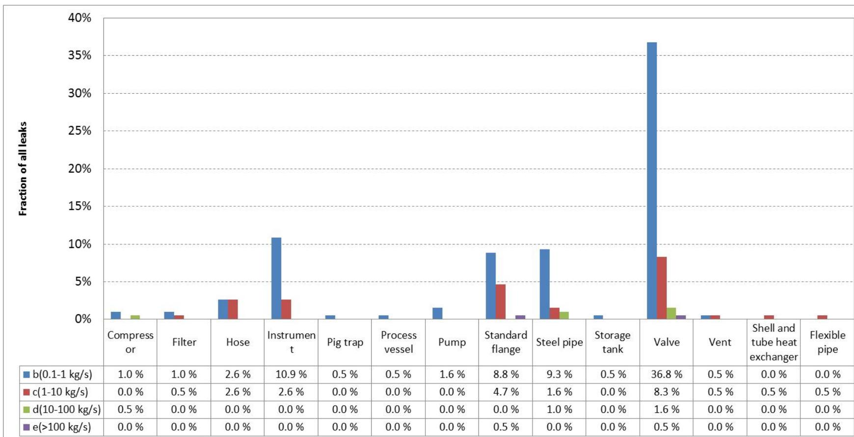
Figure 3.9 - Relative distribution of all NCS leaks (193) per equipment type where leaks stemming from equipment in open drain, closed drain, flare system, well system, produced water system and unknown systems have been disregarded (see Table 3.1)
