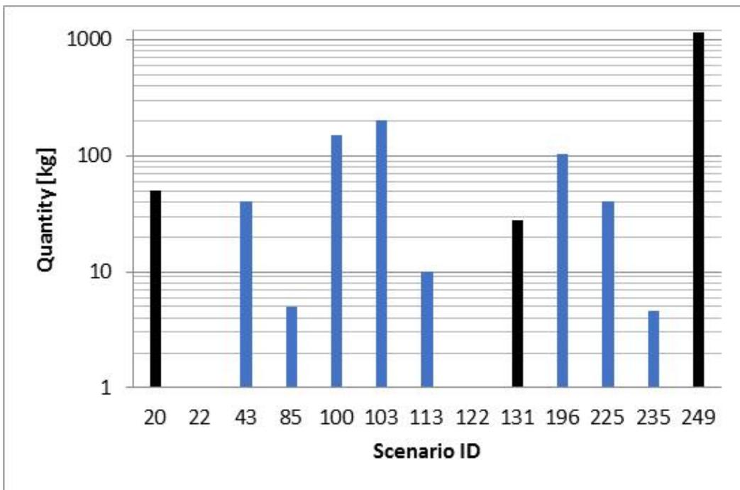
Figure 3.28 - Released quantity for hose leaks recorded on NCS 2001 – 2017. The y-axis is in logarithmic scale
