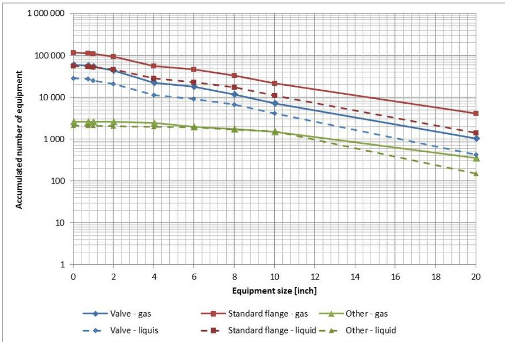
Figure 4.12 - Accumulated number of equipment versus equipment dimension (i.e. the number of leak from equipment with dimension larger than the x-value), equipment containing gas and liquid separately. All 90 installations being in operation in the period 2001 – 2017 are included. Other equipment excludes hose and instrument (and valve and standard flange) as they are all 3/4"
