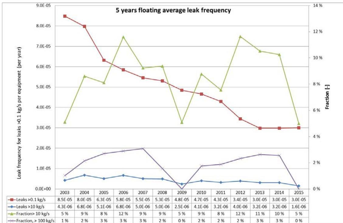
Figure 5.9 – 5 years floating average frequency for leaks  $\geq 0.1$  kg/s and  $\geq 10$  kg/s per equipment for various time periods. Floating average plotted versus the middle year of the period that is averaged (*i.e.* the data point for year 2012 applies for the period 2010-2014). Furthermore the fraction of leaks  $\geq 10$  kg/s and  $\geq 100$  kg/s is given (green and violet curve). Note that these curves are read on the right axis
