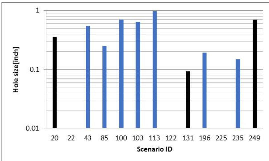
Figure 3.26 – Hole size for hose leaks recorded on NCS 2001 – 2017. The y-axis is in logarithmic scale
