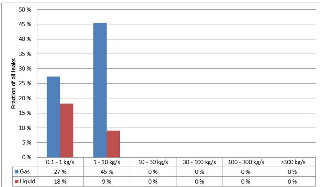
Figure 3.21 - Relative distribution of leaks from hoses with respect to initial leak rate for all Significant NCS leaks (total leaked quantity >10 kg, see TN-4) per fluid phase
