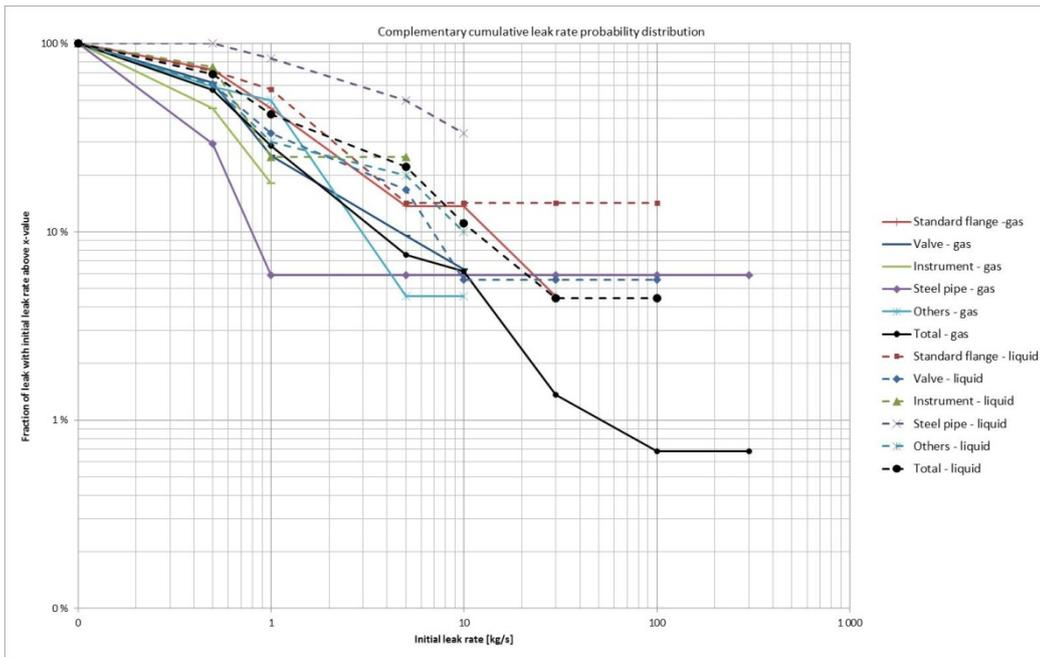
Figure 3.16 - Complementary cumulative probability distribution with respect to initial leak rate for Significant NCS leaks (total leaked quantity >10 kg, see TN-4) per fluid phase. Note that the leaks are categorized into leak rate categories. See also text above
