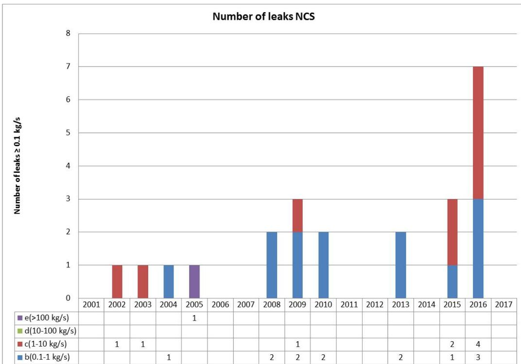
Figure 5.3 - Distribution of NCS leaks (23) versus time for installations set in operation in the period 01.01.2001 – 31.12.2017
