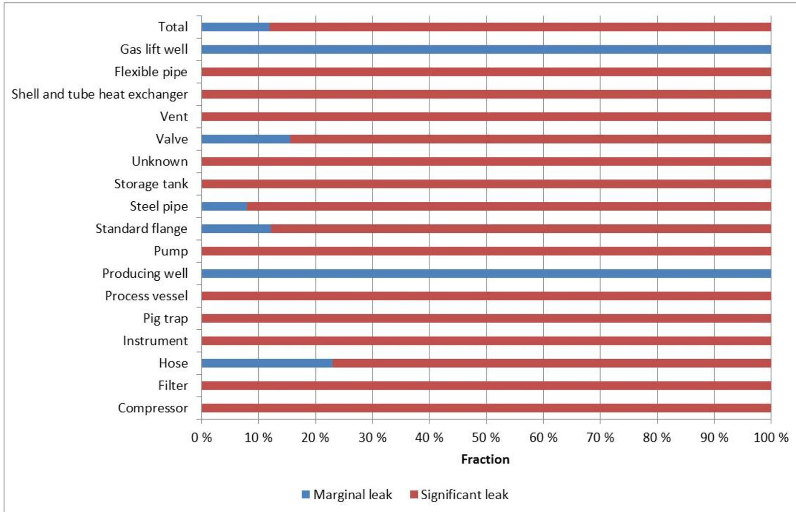
Figure 3.5 - Relative distribution of all NCS leaks (217) per leak scenario per equipment type. NB! Only two events are related to producing wells
