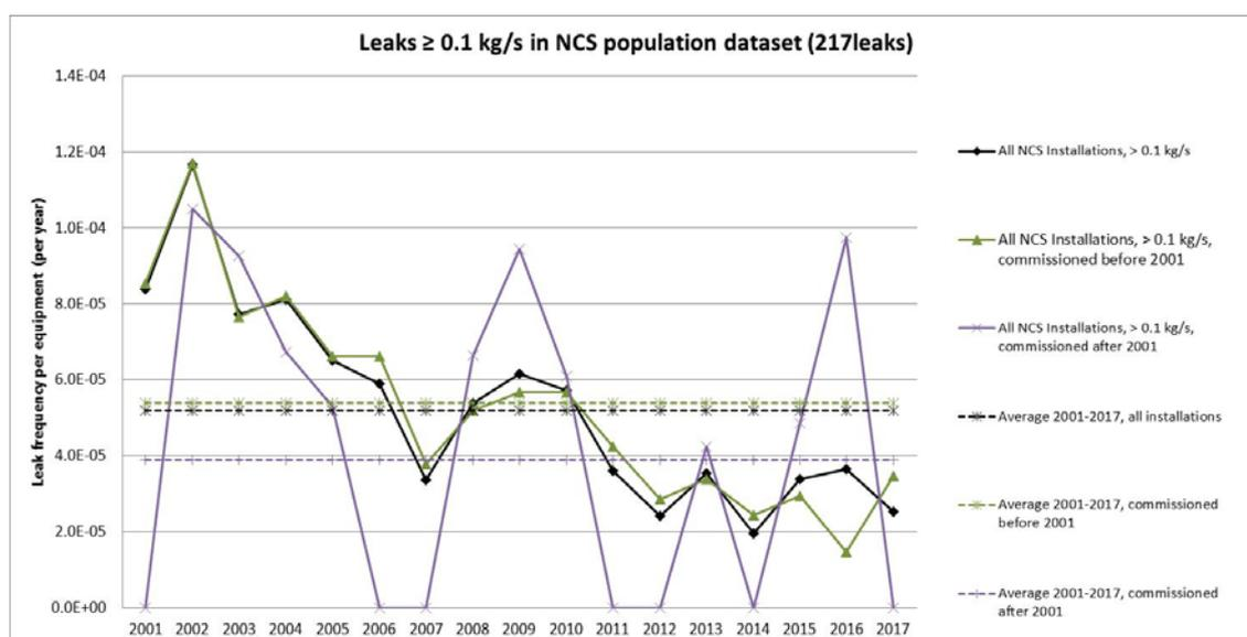
Figure 5.4 - Average frequency for leaks ( $\geq 0.1$  kg/s) per component versus time for installations in the NCS population dataset (217)
