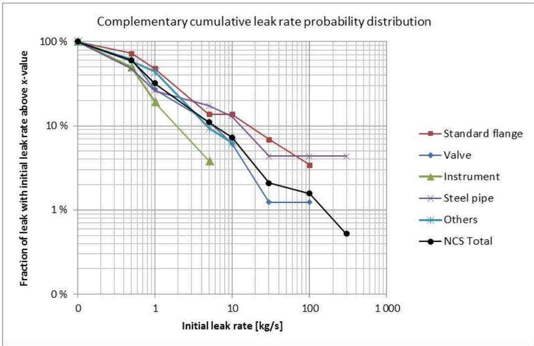
Figure 3.14 - Complementary cumulative probability distribution with respect to initial leak rate for Significant leaks on installations in the NCS population dataset. Note that the leaks are categorized into leak rate categories. See also text above
