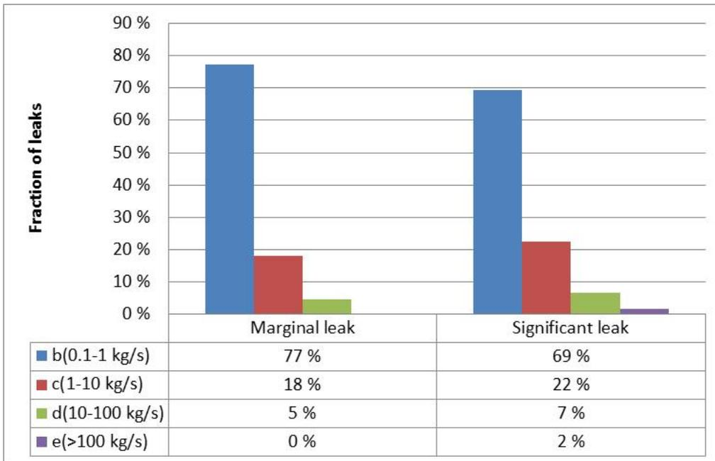
Figure 3.3 - Relative distribution of all NCS leaks (217) per leak scenario. The contributions from the initial leak rates categories sum up to 100%
