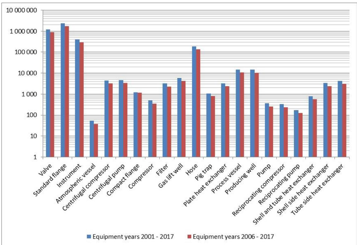
Figure 4.18 - Equipment years per equipment type in NCS population dataset in the period 2001-2017. The y-axis is in logarithmic scale
