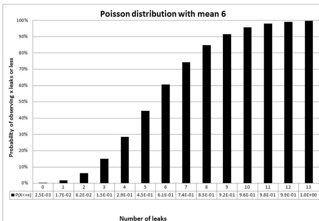
Figure 6.1 – Probability of observing x number of leaks or less with leak rate >10 kg/s, given expected number of leaks is 6
