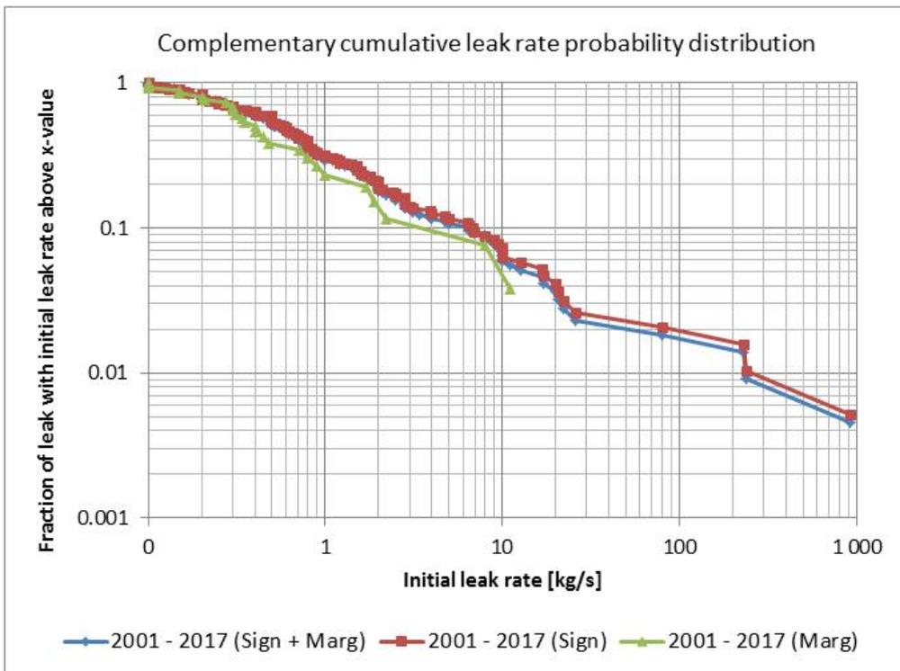
Figure 3.12 - Complementary cumulative probability distribution of NCS leaks with respect to initial leak rate both for Significant leak (total leaked quantity >10 kg, see TN-4), Marginal leak and both
