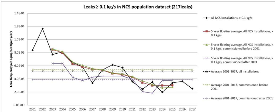
Figure 5.5 - Average frequency and floating average for leaks ( $\geq 0.1$  kg/s) per component versus time. Floating average plotted versus the middle year of the period that is averaged (*i.e.* the data point for year 2012 applies for the period 2010-2014)
