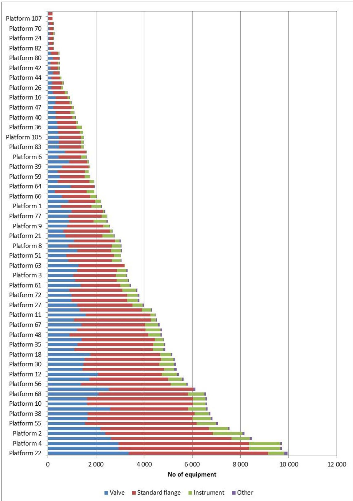
Figure 4.3 - Distribution equipment counts for dominant type of equipment (standard flange, valve and instrument) for the 90 installations being in operation in the period 2001 - 2017. Steel pipe, well and hose operations are not included as part of the category "Others"
