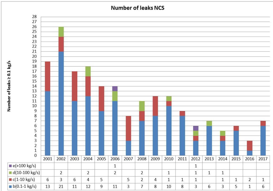
Figure 5.2 - Distribution of NCS leaks (194) versus time for installations set in operation before 01.01.2001
