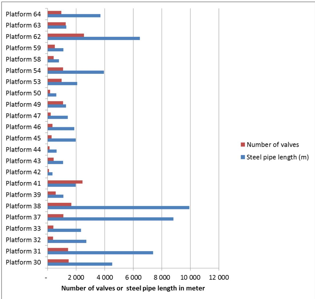
Figure 4.8 - Number of valves and steel pipe for installations where counts of steel piping is included in the NCS population dataset
