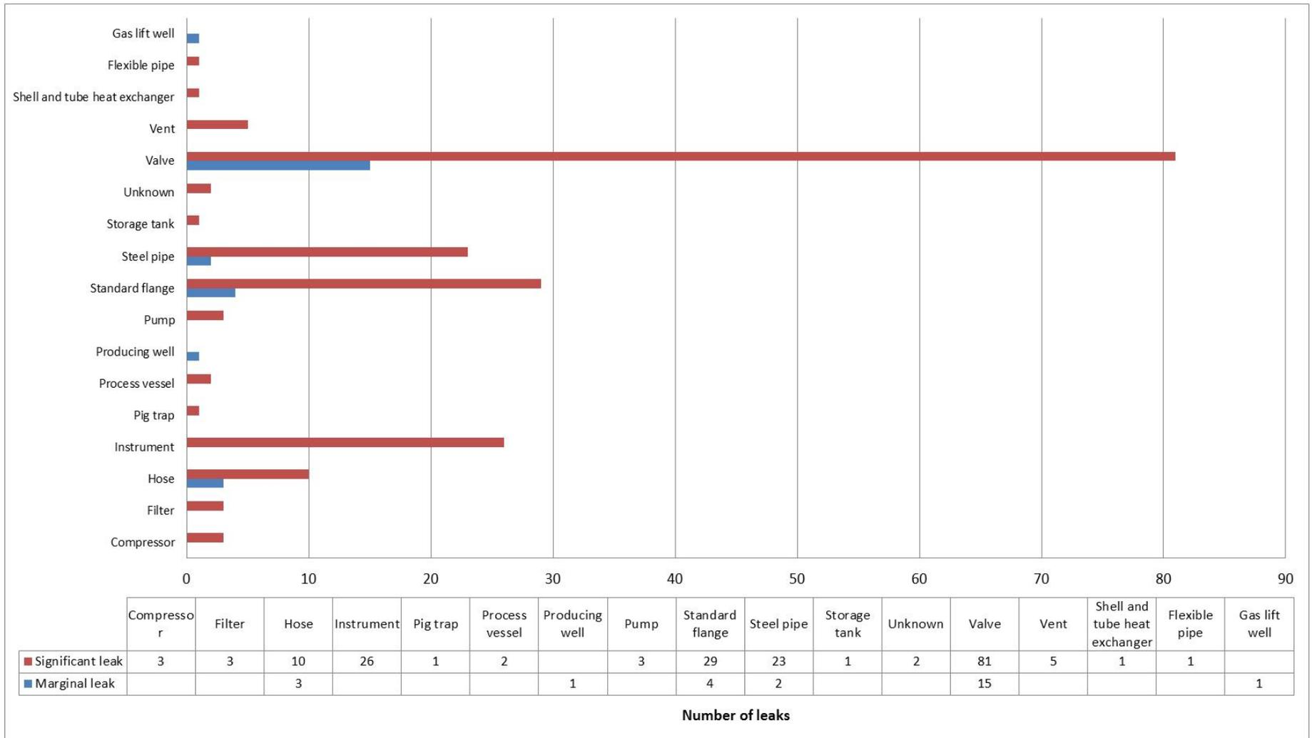
Figure 3.4 - Distribution of all NCS leaks (217) per leak scenario per equipment type
