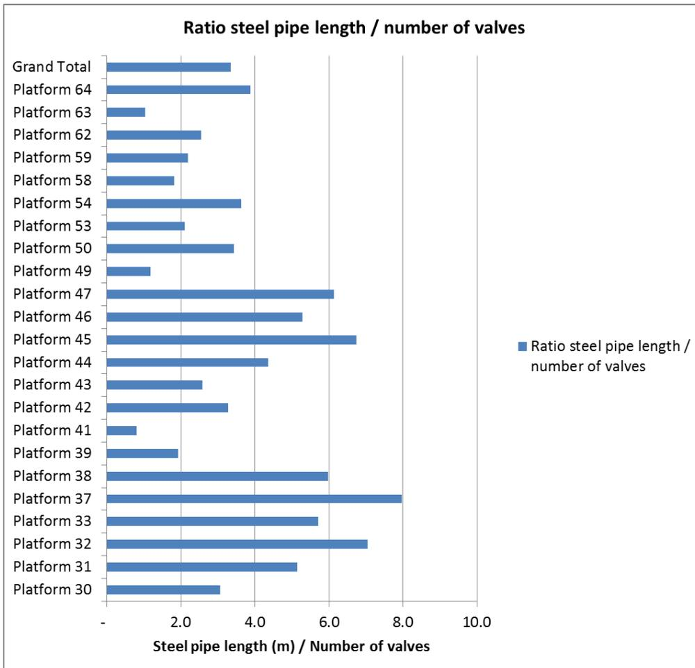
Figure 4.9 - Ratio steel pipe length divided by number of valves for installations where counts of steel piping are included in the NCS population dataset
