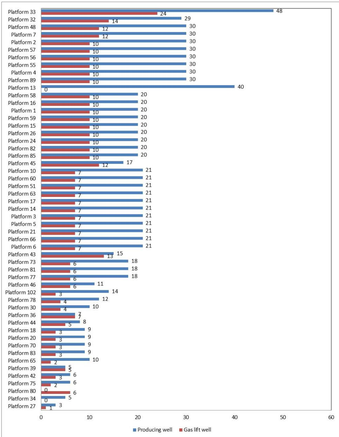
Figure 4.10 - The total number of topside producing wells (wells with and without gas lift) and the number of producing wells with gas lift on the installations in the NCS population dataset being in operation in 2001 – 2017 (90 installations). Only installations with wells are included
