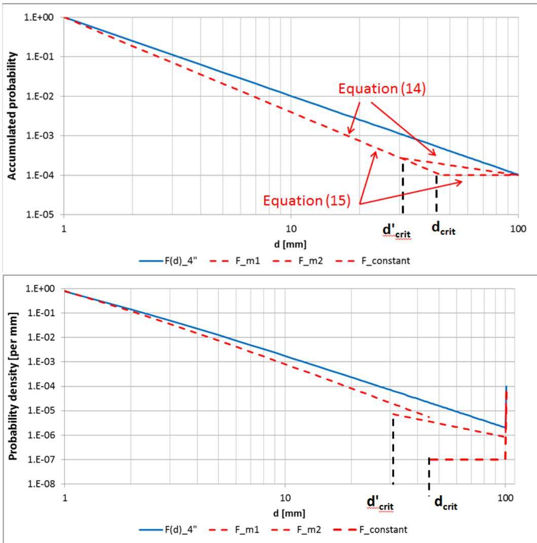
Figure 4.1 - Illustration of how the actual accumulated probability hole size distribution (above) and the probability density hole size distribution (below) might look like. The blue curve is a standard power law for a 4" equipment, while the red curves illustrate the two concepts described in equation (14) and (15) above. F\_m1, F\_m2 and F\_constant have identical line colour as they belong to the same model.
