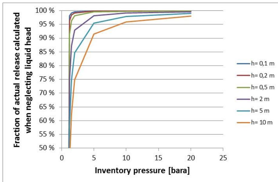
Figure 3.1 - The effect of neglecting liquid head. The figure gives the fraction of the actual leak rate calculated by neglecting the liquid head h, for a range of values for the liquid head
