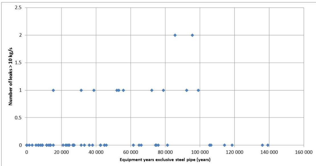
Figure 4.5 - Number of recorded leaks with initial leak rate >10 kg/s vs. recorded equipment years at installations at NCS. Note that steel pipes are not included. Each dot represents one installation
