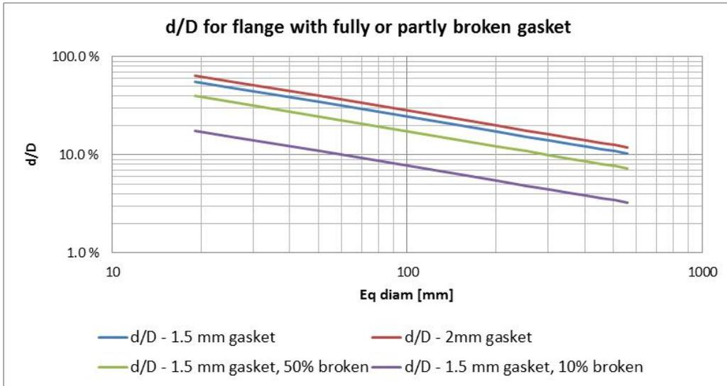
Figure 4.5 – d/D for flanges with fully or partly broken gasket. The curves could be compared with Figure 4.4, giving good reasons for arguing for a high alpha value for flanges with gaskets
