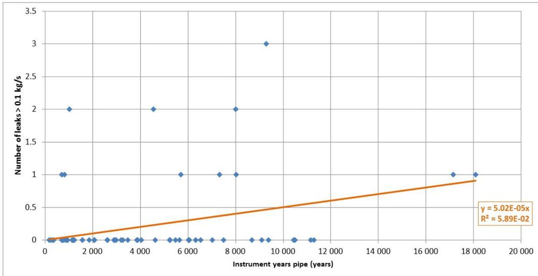
Figure 4.4 - Number of recorded leaks from Instruments with initial leak rate >0.1 kg/s vs. recorded instrument years at installations at NCS
