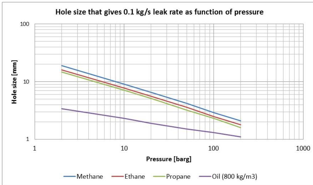
Figure 2.1 - Hole size that gives 0.1 kg/s leak rate as function of gauge pressure for Methane, Ethane, Propane and oil with density 800 kg/m<sup>3</sup>
