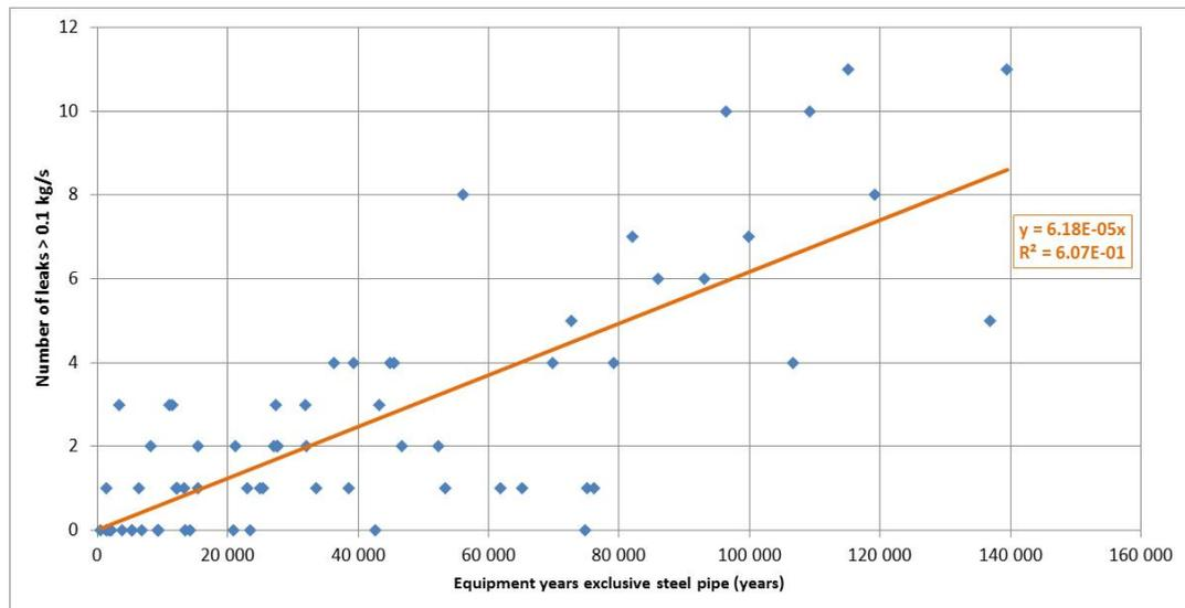
Figure 4.1 - Number of recorded leaks with initial leak rate >0.1 kg/s vs. recorded equipment years at installations at NCS. Note that steel pipes are not included. Each dot represents one installation
