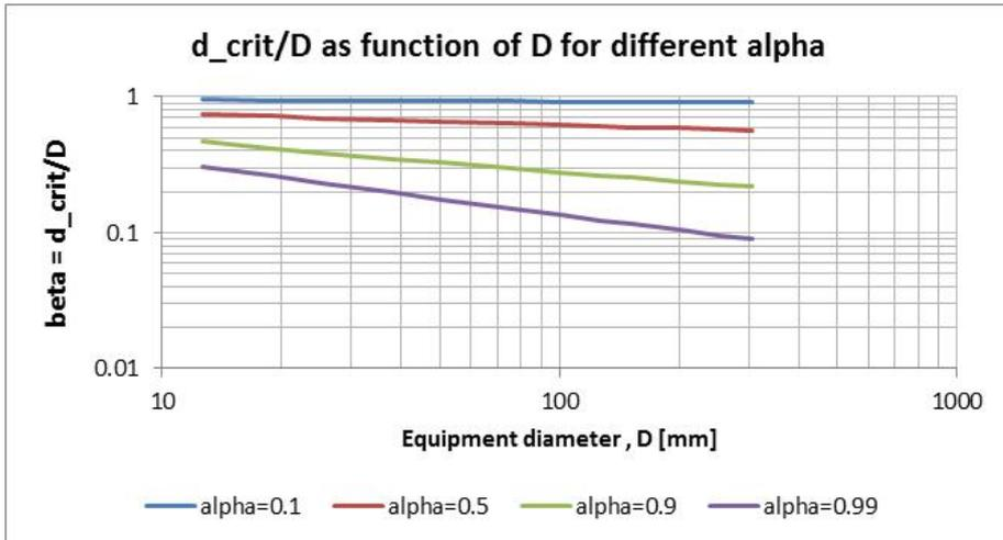
Figure 4.4 -  $\beta = \frac{d_{crit}}{D}$  as function of equipment diameter,  $D$ , for different values of
