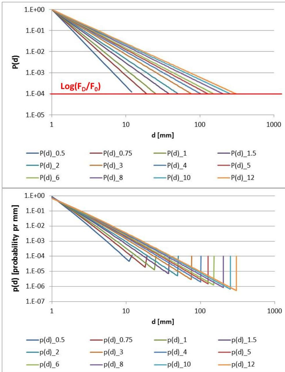
Figure 3.3 - Above: Illustration of the hole size probability distribution, given by  $F(d)/F_0$ , for a range of equipment diameters (the legend gives the dimension in inches). Below: The underlying hole size probability density distribution
