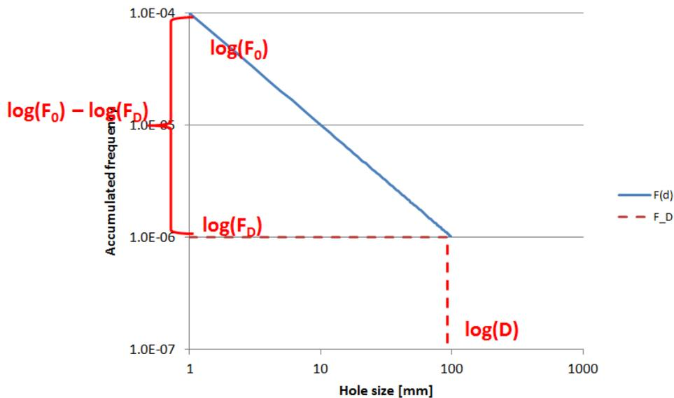
Figure 3.2 - Illustration of the slope parameter,  $m$  for a 4 inch equipment
