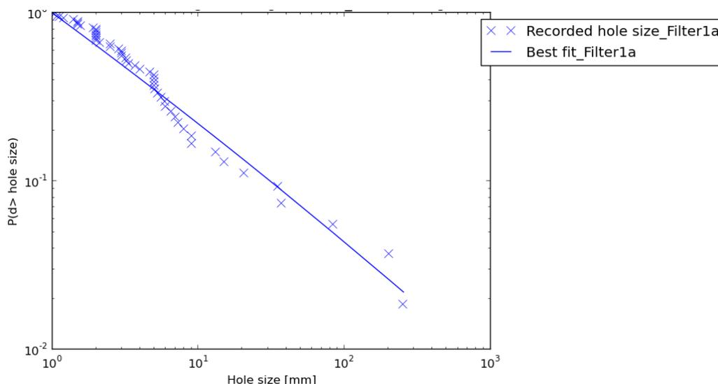
Figure 2.1 - Curve fitting to recorded HCRD hole size distribution for Standard flange (Medium size: 3-11"). The data shows a power law behaviour
