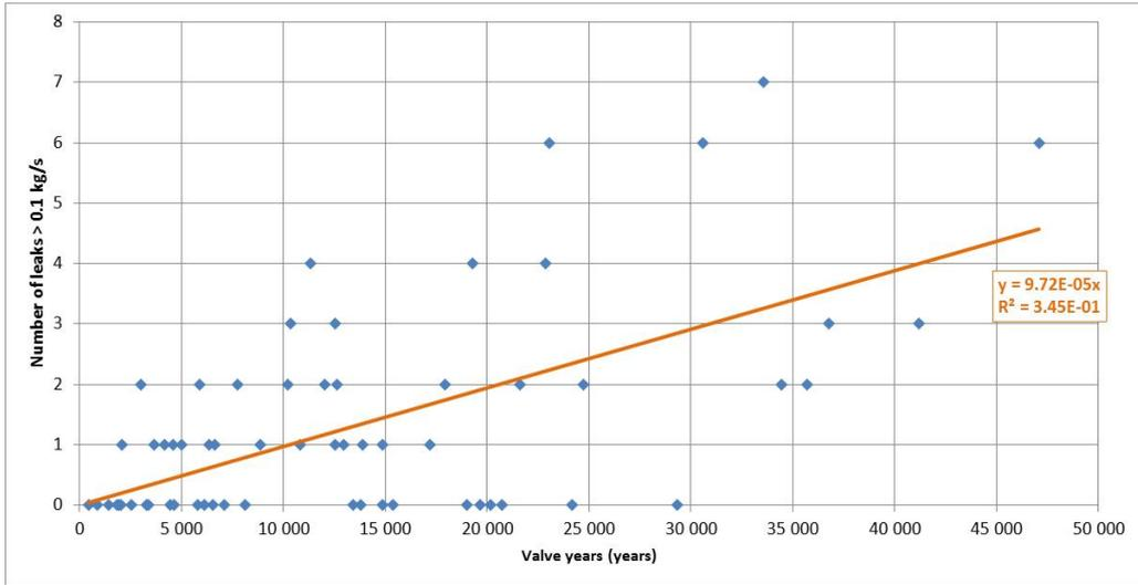
Figure 4.2 - Number of recorded leaks from Valves with initial leak rate >0.1 kg/s vs. recorded valve years at installations at NCS
