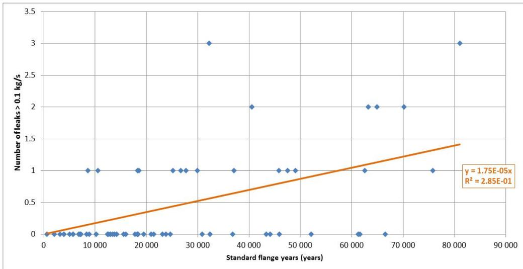
Figure 4.3 - Number of recorded leaks from Standard flange with initial leak rate >0.1 kg/s vs. recorded Standard flange years at installations at NCS
