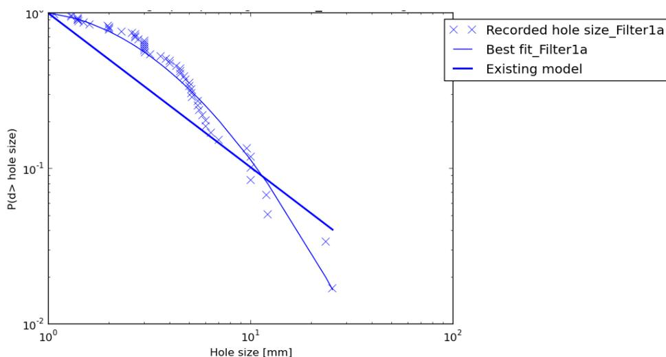
Figure 2.2 - Curve fitting to recorded HCRD hole size distribution for centrifugal compressor. A better fit is achieved using equation (2) for the slope parameter,  $m$  (thin blue curve), than by assuming a constant slope parameter (thick blue curve),  $m$ . Existing model refers to the SHLFM, Ref. /2/
