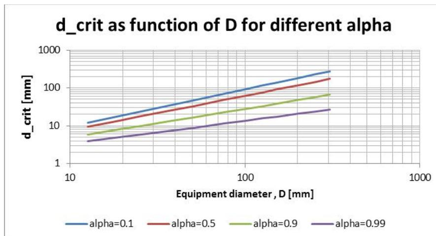
Figure 4.3 -  $d_{crit}$  as function of equipment diameter,  $D$  for different values of  $\alpha$
