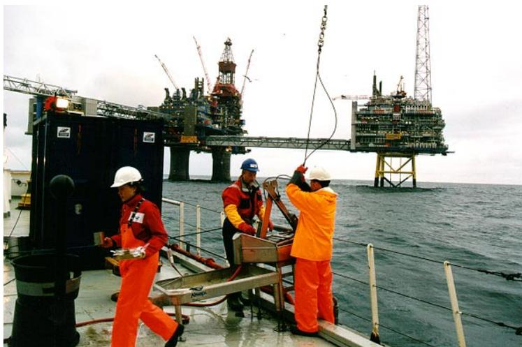
*A sediment sample being brought aboard with the van Veen grab.*
