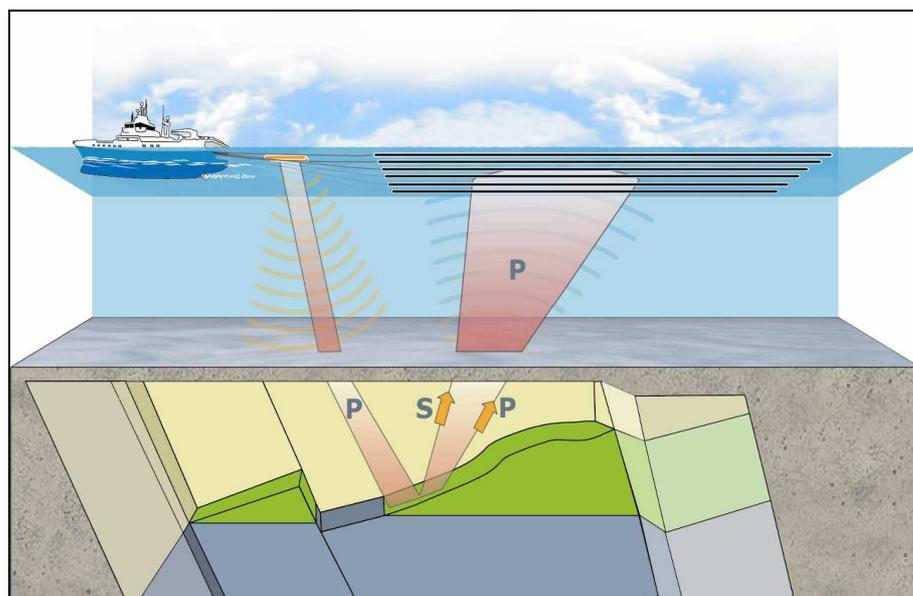
**Figure 3-2.** Schematic diagram for 3D seismic. Multiple listening cables and at least one sound source are used. (Figure © Statoil).
