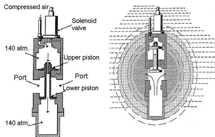
**Figure 3-3.** Sketch of a Bolt-PAR air gun cross-section before firing and after firing. Figure obtained from <http://www.bolt-technology.com>
