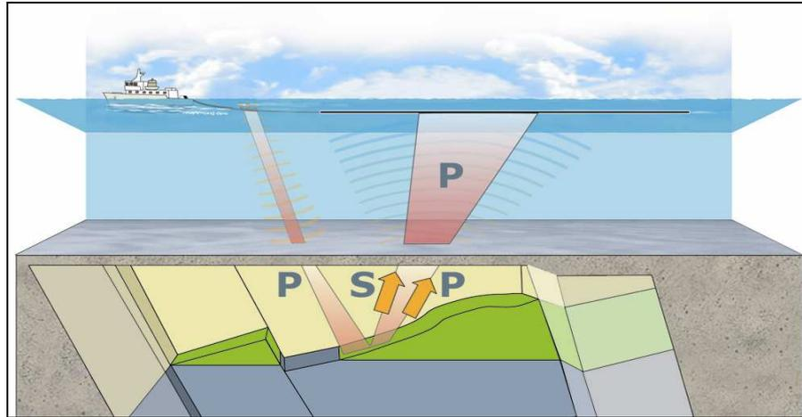
**Figure 3-1.** Schematic diagram for 2D seismic. The vessel tows a sound source and a receiver cable with hydrophones. P = pressure waves, S = shear waves (Figure © Statoil).
