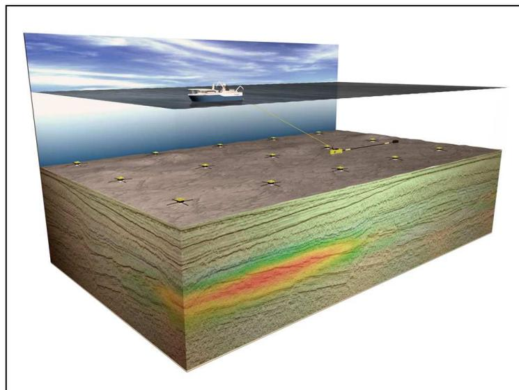
**Figure 3-4.** Schematic diagram for electromagnetic surveys. The vessel tows a low-frequency electromagnetic source in deep water. Reflected signals are captured by a number of receivers placed on the seabed.
