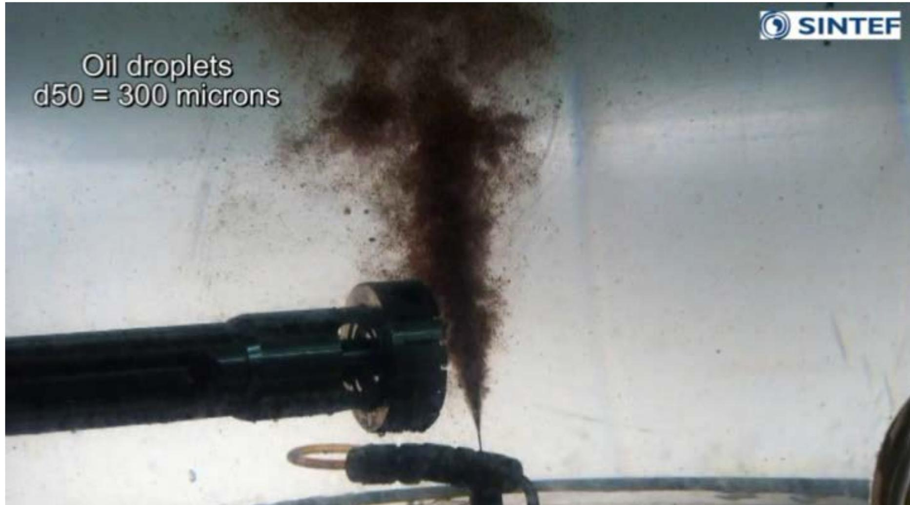
The mechanical shearing device used in the MiniTower (80 liters of natural sea water)
