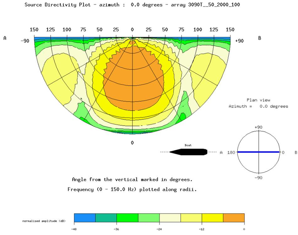
Figure 3.12. Relative directivity diagram along ship. The numbers along the abscissa axis (A-B) indicate frequencies as the directivity response of a given source at a certain angle is frequency dependent. (Schoolmeesters, 2002).
