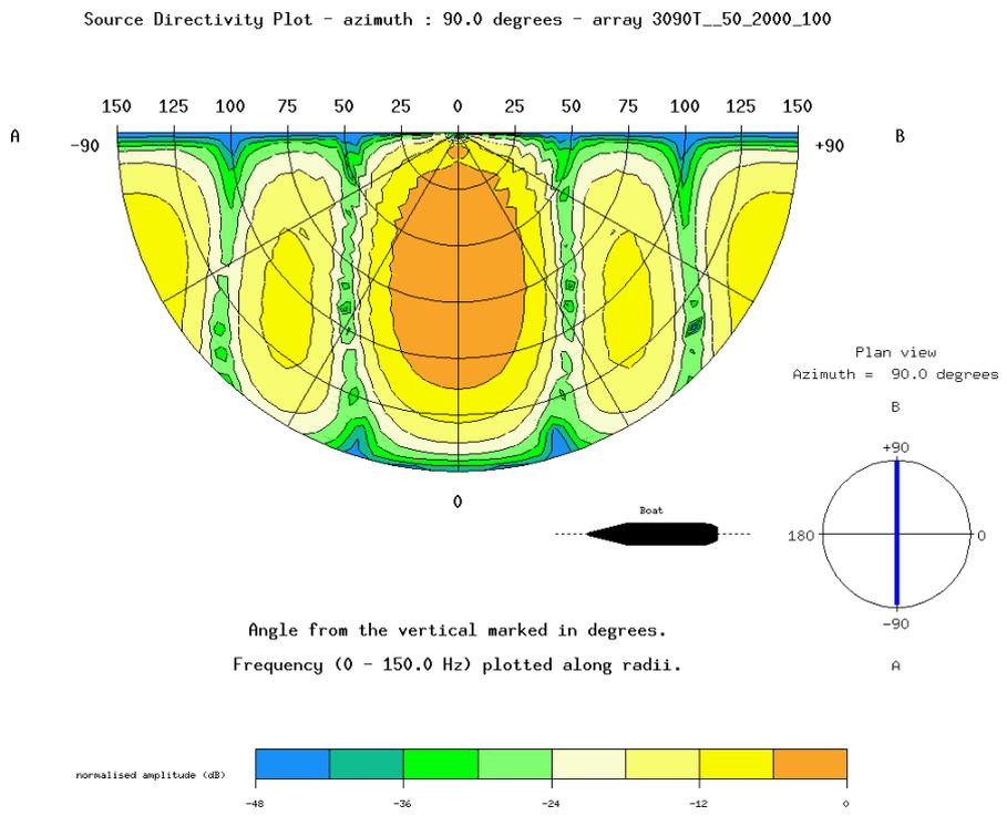
Figure 3.13. Relative directivity diagram of the pressure distribution athwart ship. The numbers along the abscissa axis (A-B) indicate frequencies as the directivity response of a given source at a certain angle is frequency dependent. (Schoolmeesters, 2002).
