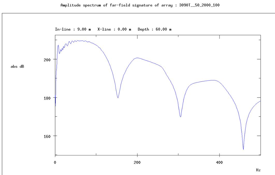
Figure 3.11. Amplitude-frequency spectrum of the pressure signature of Figure 3.13 (Schoolmeesters, 2002).
