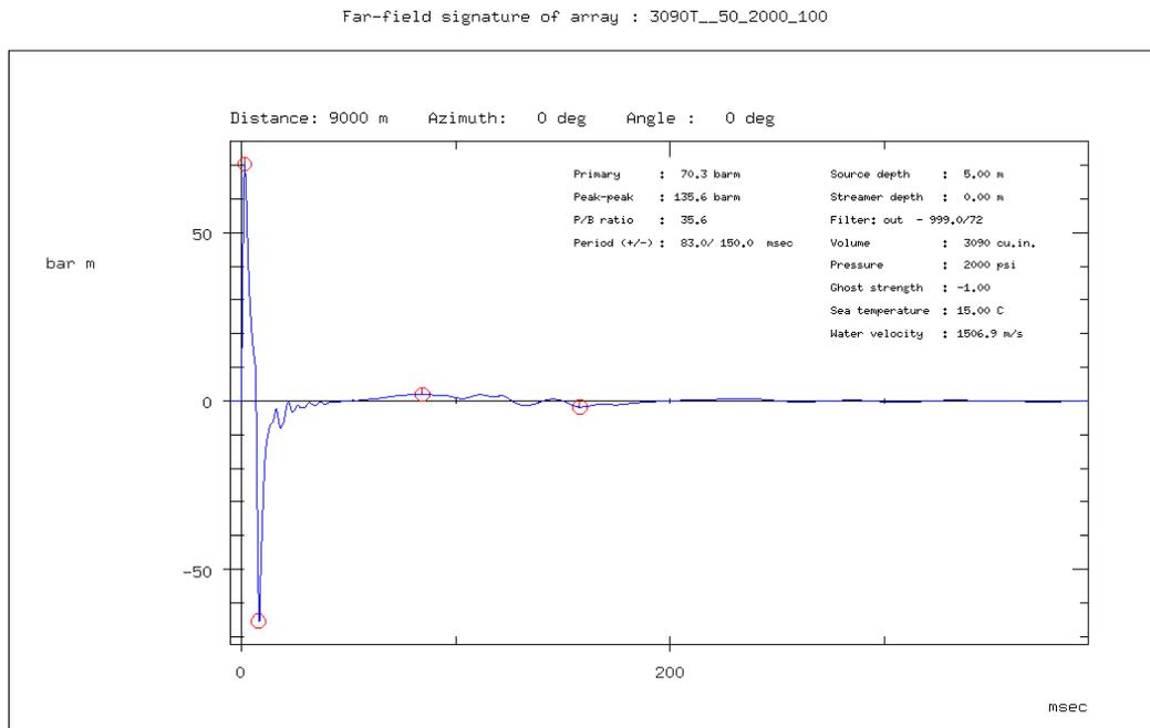
Figure 3.9. Far field pressure signature from the airgun array in bar m (pressure in bar referred to 1 m from the source centre) versus time [ms] (Schoolmeesters, 2002).
