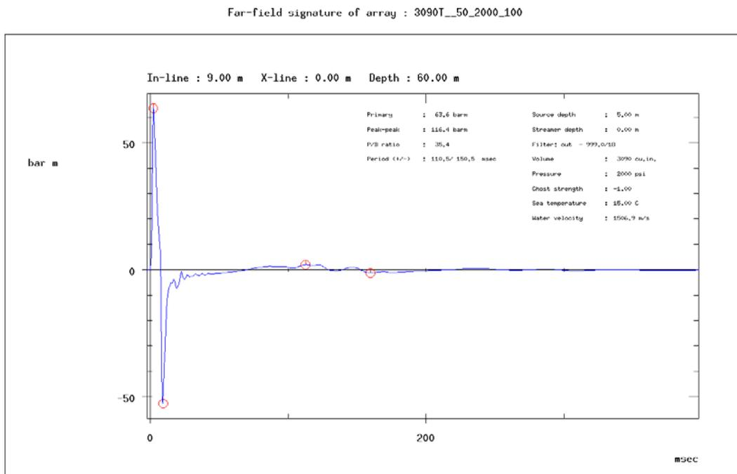
Figure 3.10. Near field pressure signature from the airgun array in bar m (pressure in bar referred to 1 m from the source centre) versus time [ms]. Measurement position is  $x = 9.0$  m  $y = 0.0$  m, and depth,  $z = 60.0$  m which means vertically underneath the centre of gravity of the array (Schoolmeesters, 2002). (Note: PGS' "NUCLEUS" expresses this as "far-field signature").
