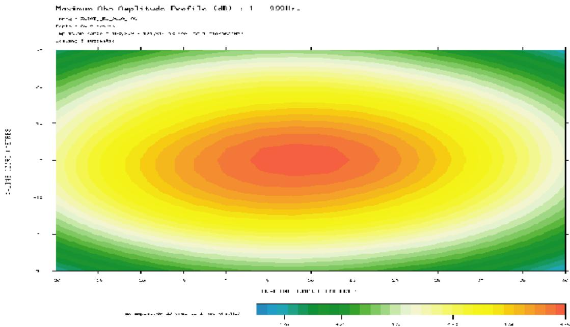
Figure 3.14. Sound pressure as maximum absolute amplitude profile distribution at the bottom at 60 m depth for the frequency range 1-999 Hz. Covered extension area is 60x60 m right below the airgun array which centre being at coordinates 0,0.
