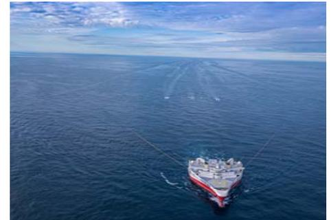
*Exploration seismic survey with Ramform vessel.*
