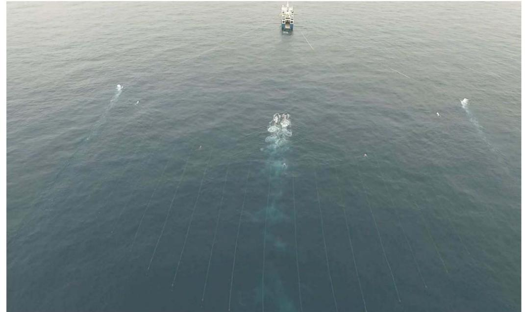
*P-cable with 18 x 100m x 12.5m streamer spread and dual source (Wisting, 2016)*
