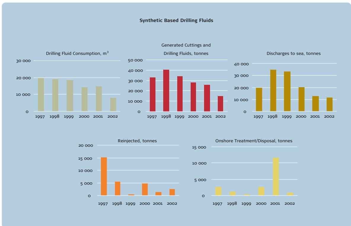
Figure 6 – Disposal of drilling waste from using synthetic fluids for the years 1997-2002.
