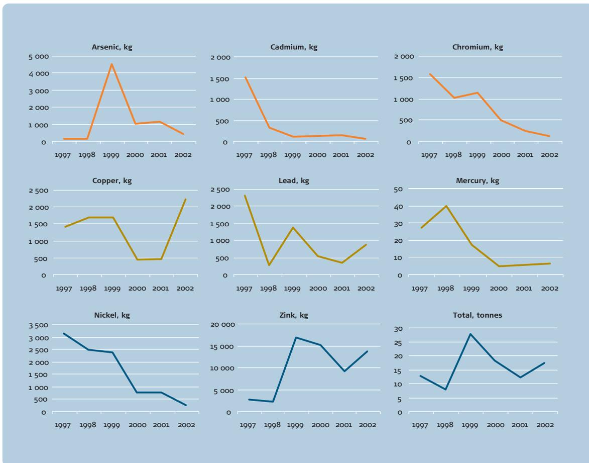
Figure 10 – Heavy metals discharged with produced water.
