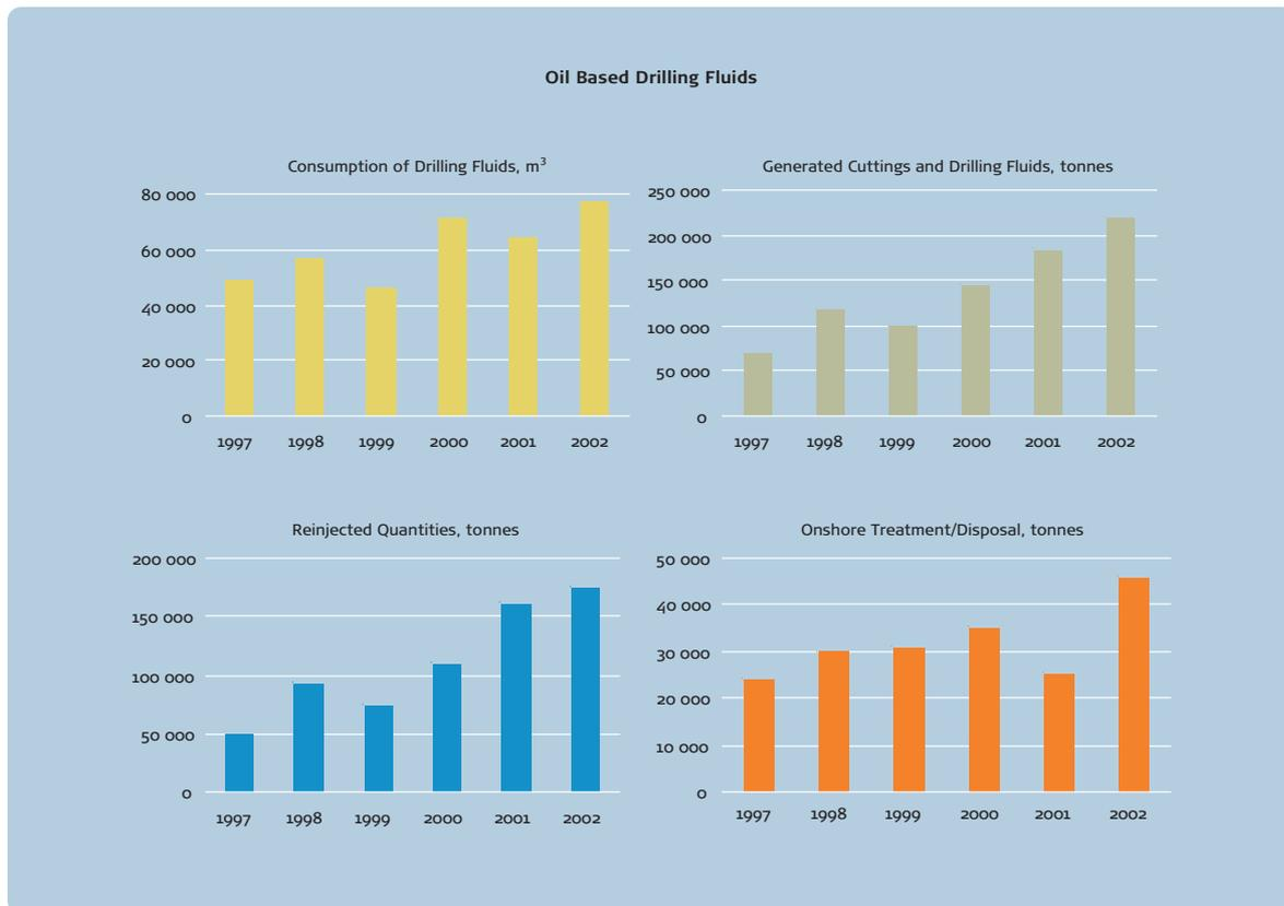
Figure 5 – Key figures from drilling with oil based drilling fluids for the years 1997-2002.
