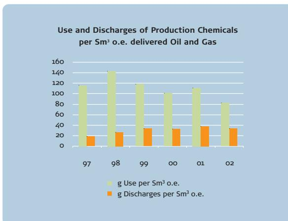
Figure 14 – Use and discharges of production chemicals per Sm³ o.e. oil and gas.
