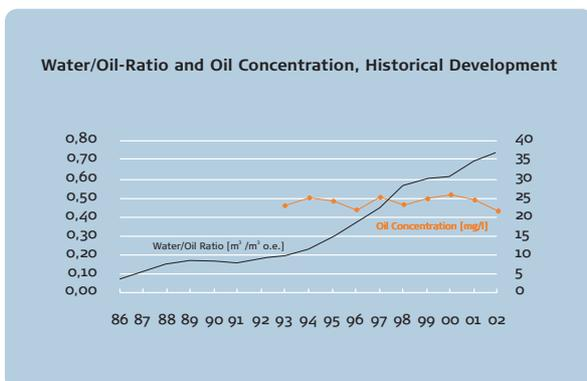
Figure 9 – The historical development of the relation between produced quantities of water and oil (left scale). Right scale: Average oil concentration in produced water discharges 1993-2002.
