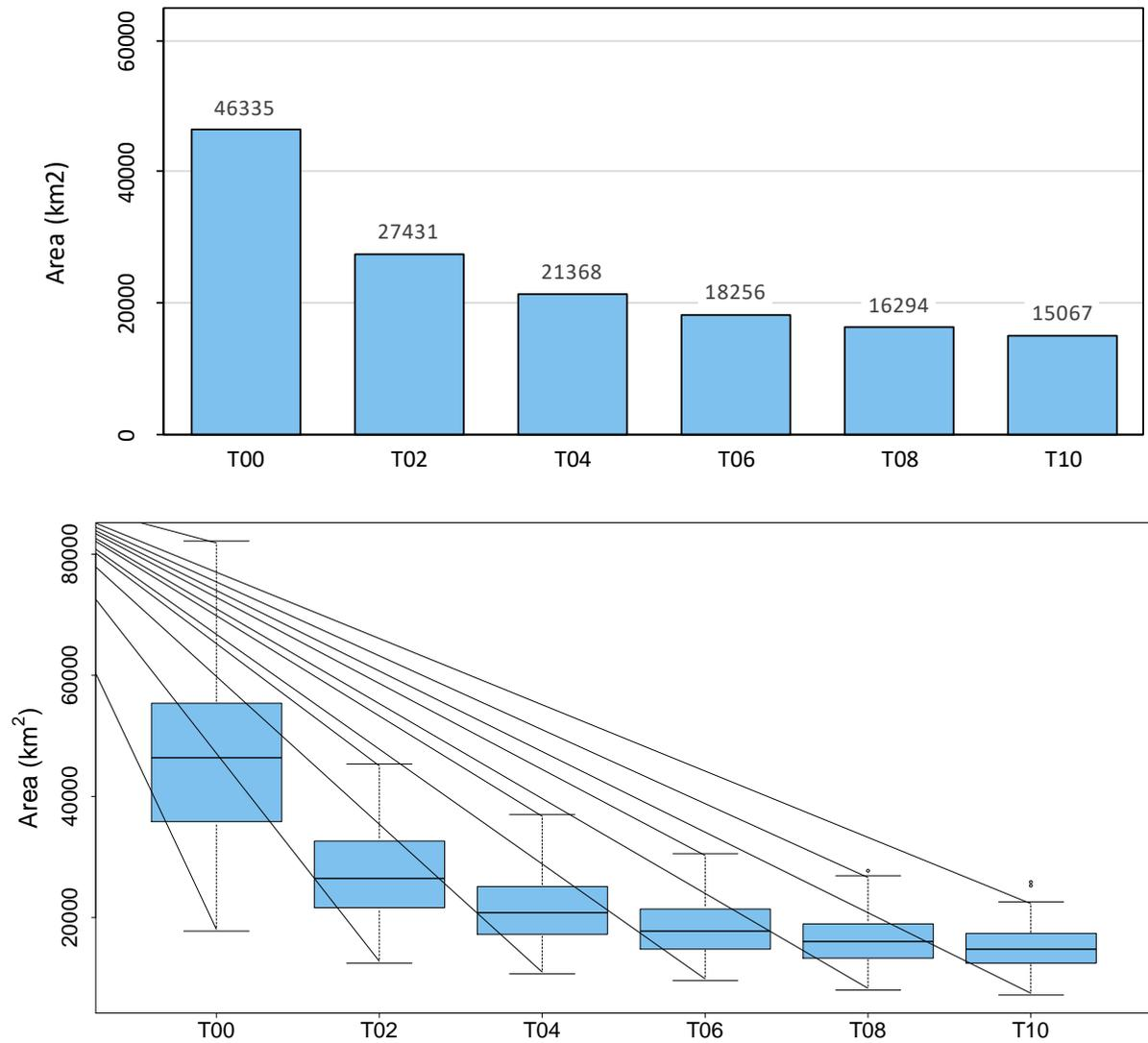
Figure 3. Column plots (top) and box plots (bottom) comparing the sea surface area above the threshold thickness (T) for the six scenarios each represented with 237 simulations. The column plot shows the mean values while the box plot illustrates the minimum, first quartile, median (typical value), third quartile, and maximum for the 237 simulations. The whisker length is set at 1.5 times the inter-quartile range (IQR), with black rings showing outliers, including minimum and maximum values.
