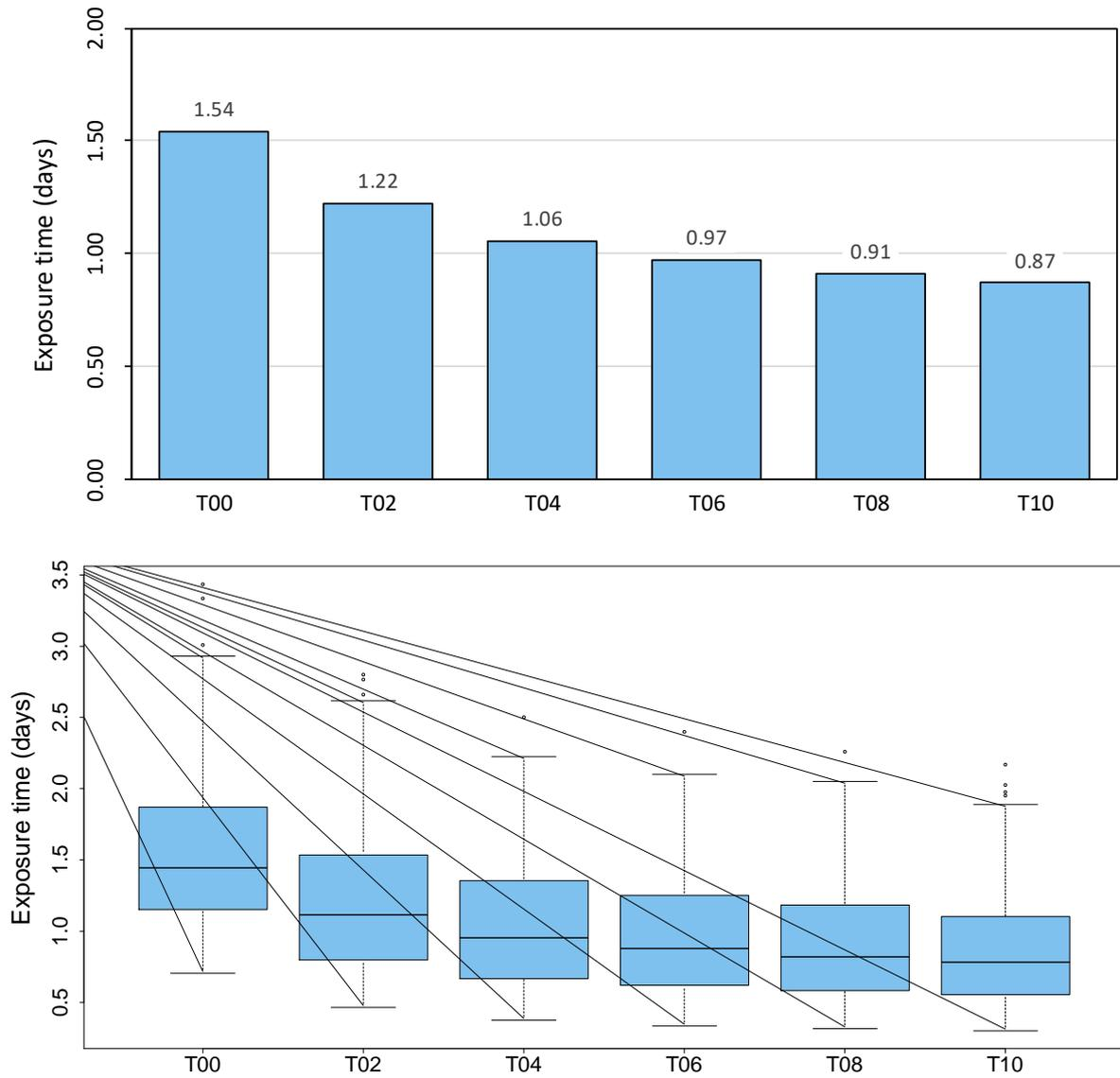
Figure 4. Column plots (top) and box plots (bottom) comparing the exposure time above the threshold thickness (T) for the six scenarios each represented with 237 simulations. The column plot shows the mean values while the box plot illustrates the minimum, first quartile, median (typical value), third quartile, and maximum for the 237 simulations. The whisker length is set at 1.5 times the inter-quartile range (IQR), with black rings showing outliers, including minimum and maximum values.
