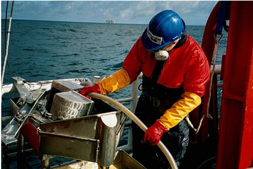
Figure 4 Sampling on the Norwegian shelf showing the Van Veen grab being rinsed. Photo: Hans-Petter Mannvik
