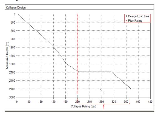
Fully evacuated Bannulus – loads exceeded with 180 bar, not accounted for wall loss
