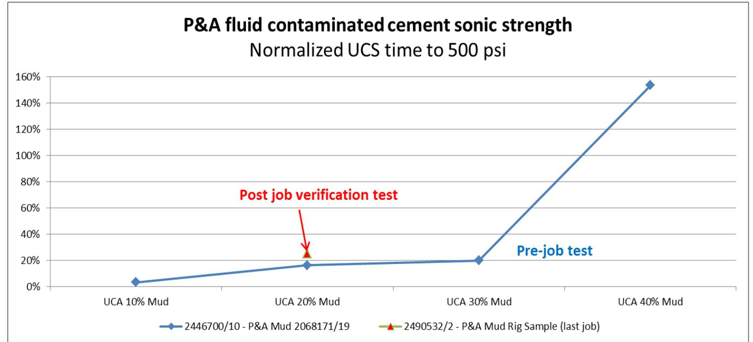
A heavily diluted cement will not have the necessary low permeability to be a barrier
