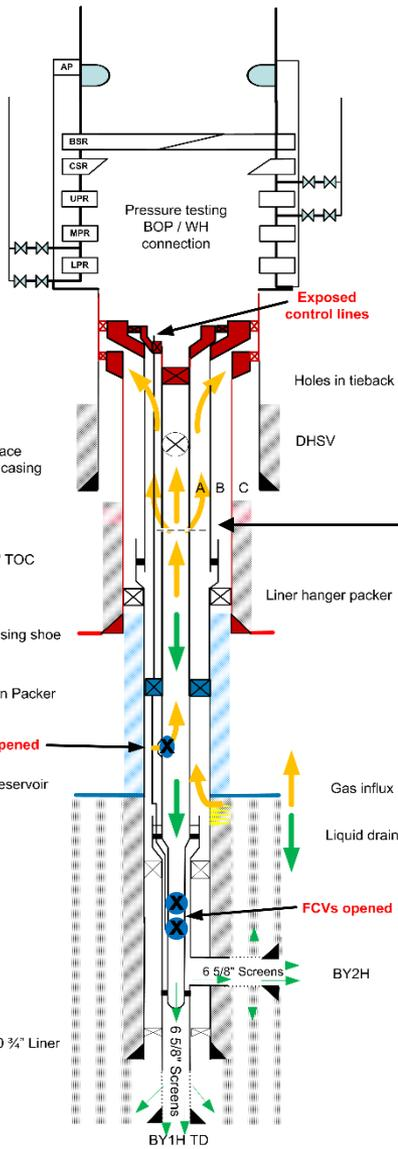
BOP/WH connector test. **Exposed control lines** for gas-lift valve (GLV) and flow control valves (FCV).
