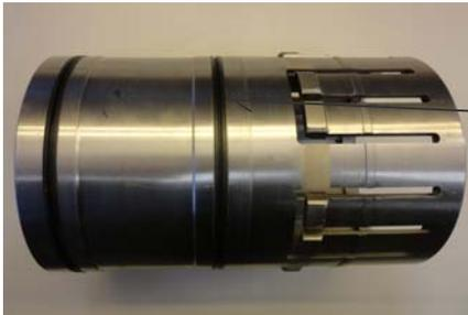
O-rings on sliding sleeve were leaking
