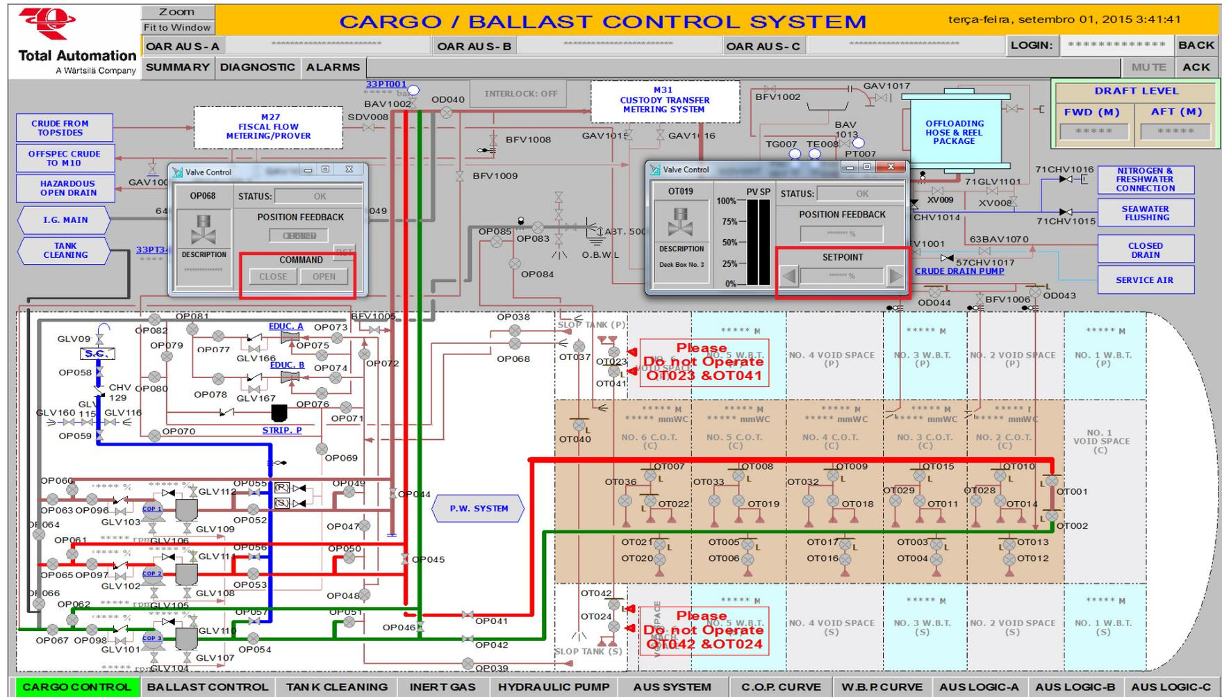
Figure 59 – Windows pop up in the HMI supervisory system for operating the valves
