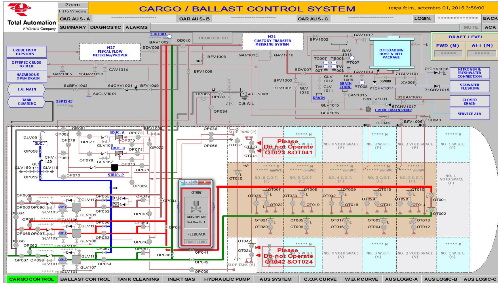
Figure 8 – Windows pop up in the HMI supervisory system for controlled valves outward CCRM.
