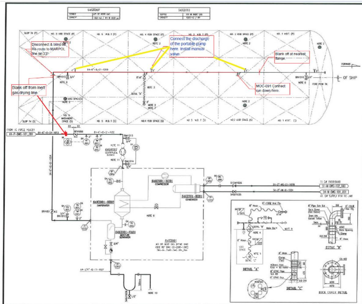
Figure 77 - P & ID with connection of submersible pumps with temporary line
