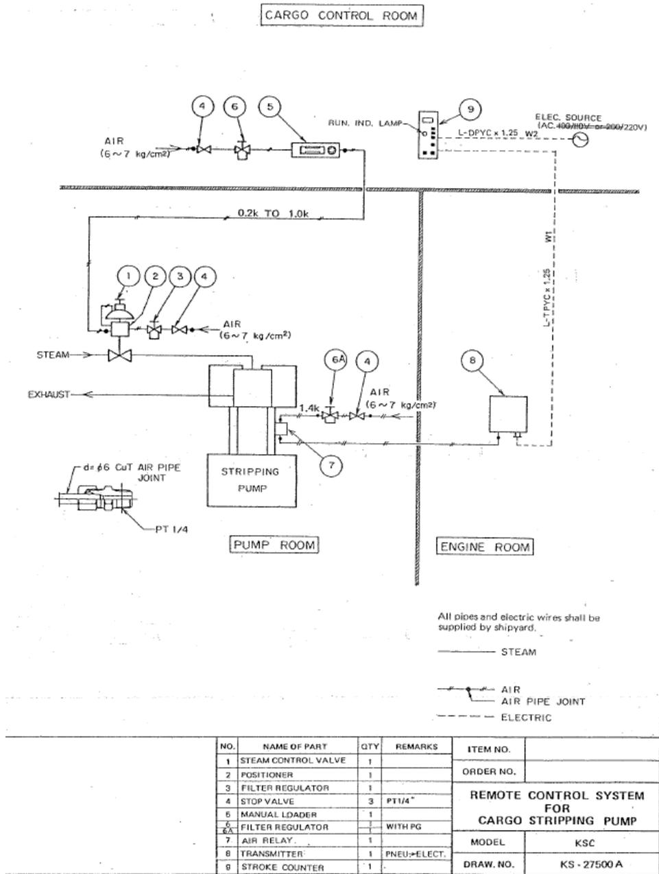
Figure 63 - Control scheme of the stripping pump
