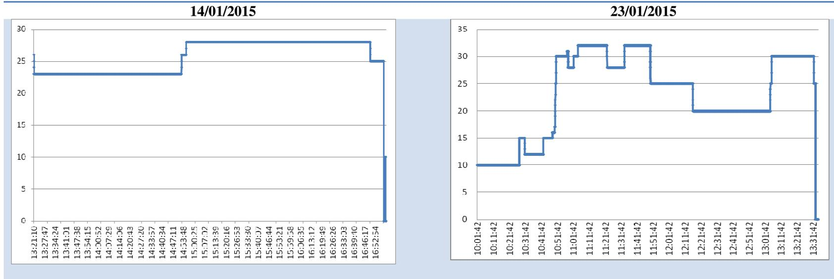
Figure 115 - Steam Flow charts for the stripping pump
