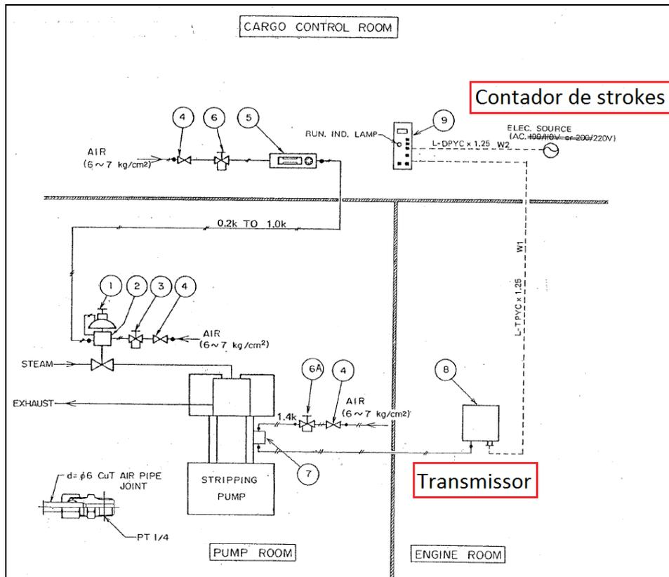
Figure 118 - Wiring diagram between the stripping pump and the CCR for the transmission of strokes count
