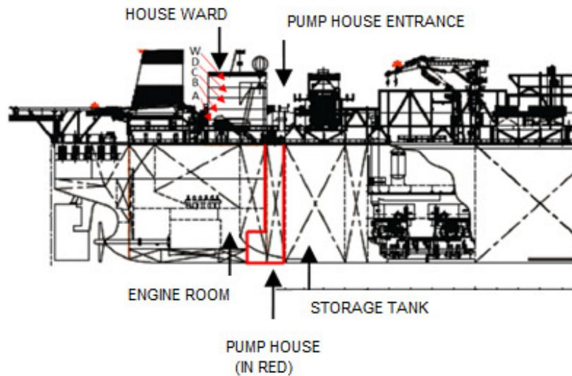
Figure 4 - Location of the pumps room and engine room
