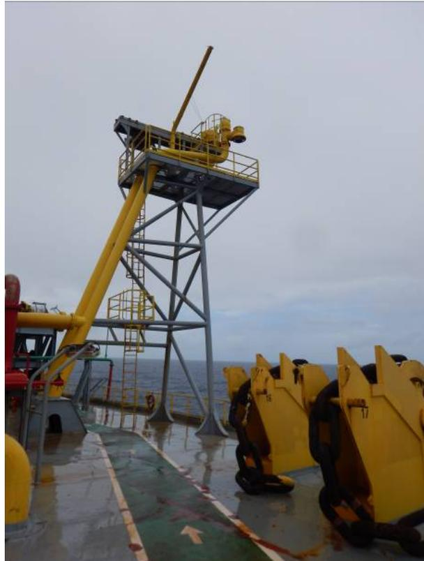
Figure 94 - Vent riser, the ship's starboard side
