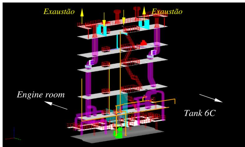
Figure 50 – Representation of exhaustion in the pumps room
