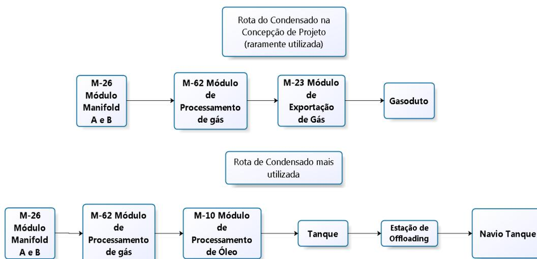
Figure 99 - condensate simplified processing route from gas
