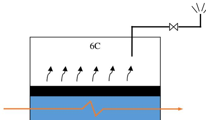
Figure 95 - Simplified scheme condensate vaporization operation
