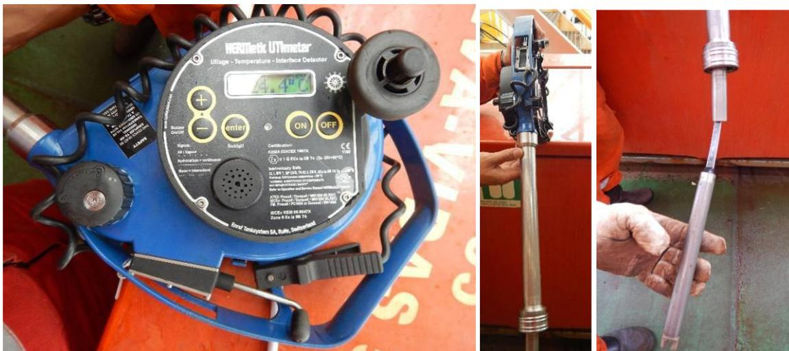
Figure 67 - Photos front and side of the ICU meter
