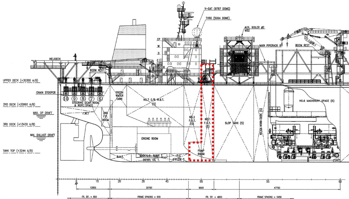
Figure 48 - Position of the pumps room
