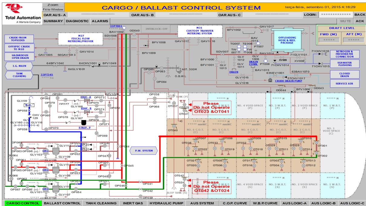
Figure 54 - IHM screen of the Supervisory System in the CCRM
