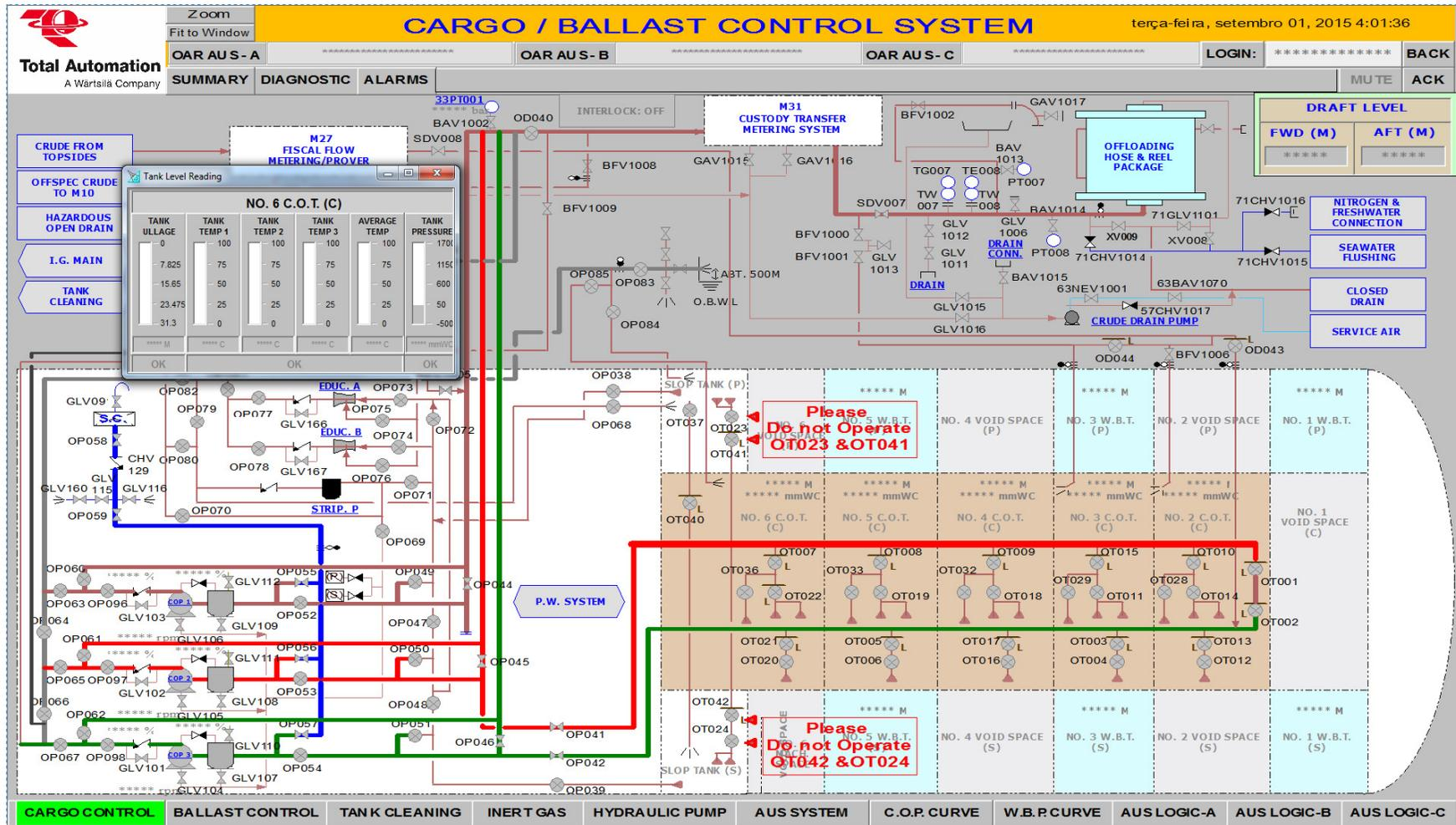
Figure 61 - Windows pop up in the IHM supervisory system for central tanks.
