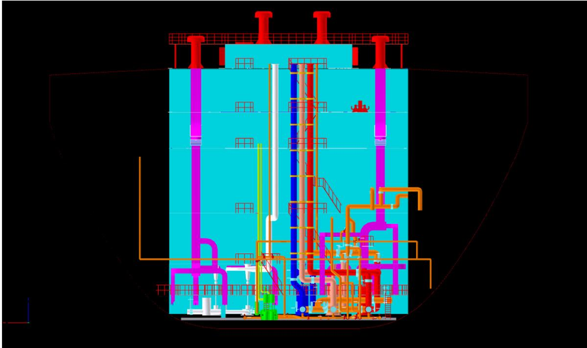
Figure 5 – *Stripping pump (green) at the inside of the cargo door*
