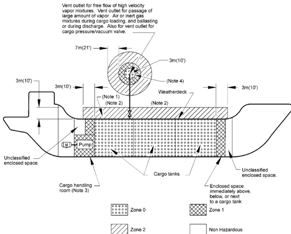
Figure 52 - Typical Area Classification for FPSOs as per API RP 505
