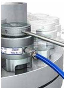
Alternatively, the tool may be installed as described under the assembly. Pressurize the tool slowly until the bolts loosen.
