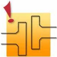
Flanges that are parallel-shifted should always be aligned before tightening can begin.
