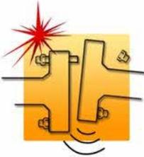
During disassembly, never assume that the line is depressurized. All flanges should be disassembled as if there is pressure in the system. The pressure build-up can occur for several reasons.
