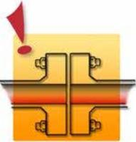
During disassembly, never assume that the line is depressurized. All flanges should be disassembled as if there is pressure in the system. Pressure build-up can arise for several reasons.
