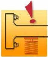
Check that the spring-loaded pipe supports are unloaded and placed in a locked position.
