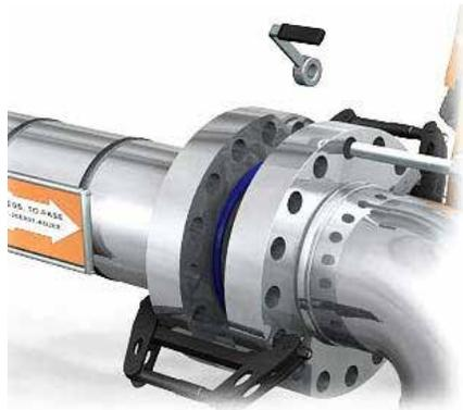
5. Keep the lowest bolts to prevent the sealing ring from falling out.
