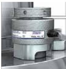
Assemble the tool with a 3 mm light opening between the wrench and the cylinder.
