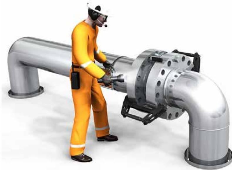
Immediately after the flanges are disassembled and cleaned, they should be inspected. Inspection personnel may need to be called in to perform a visual inspection of pipe/equipment and measure the ring track. If there is damage, this should be reported to a technical supervisor. Any tension in the pipe system should be reported to a technical supervisor.
