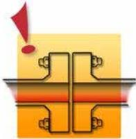
During disassembly, never assume that the line is depressurized. All flanges should be disassembled as if there is pressure in the system. Pressure build-up can arise for several reasons.
