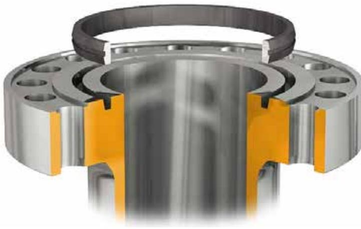
Metal-to-metal sealing ring deformation is checked. The sealing force between ring and ring track is not affected by dynamic forces since the tension in the bolts is taken up by the flange surface. This contributes to a static connection with nearly no flange movement, even when large dynamic forces are transmitted. This eliminates the need for post tightening of the bolts.
