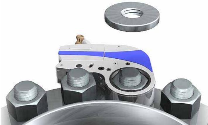
When working on flanges, where there is a need to grip or hold onto the tool, a locking disk should be installed to prevent clamp damage. For example where the tools have to be installed on the underside of the flange.
