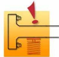
During disassembly, never assume that the line is depressurized. All flanges should be disassembled as if there is pressure in the system. Pressure build-up can arise for several reasons.
