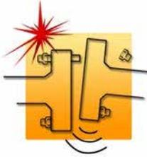
If there is tension in the pipe system that requires greater force to bring the flanges parallel to each other than the force described in the procedure below, this shall be approved by a technical supervisor for evaluation of risk and any corrective measures.
