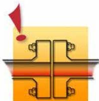
During disassembly, never assume that the line is depressurized. All flanges should be disassembled as if there is pressure in the system. The pressure build-up can occur for several reasons.
