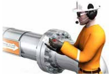
If it is necessary to use force beyond what is specified in “Alignment” to align the flange before normal tightening procedures can be started, this should be stated in the marking field in “Activity and inspection schedule” by the technician doing the work. This applies to all types of flange and clamp connections. The deviation should be recorded in the company’s system for handling deviations.
