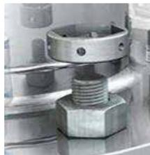
3. Check the tool size with a bolting table.
