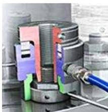
Pressurize the tool slowly until the nut can be unscrewed from the bolt. Turn the nut a 1/2 time around. Repeat the operation until all of the nuts are loosened.
