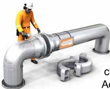
Immediately after the connection is disassembled and cleaned, it should be inspected. Additional inspection
