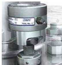
5. Assemble the wrench cap. The tool is installed on each bolt around the entire flange.
