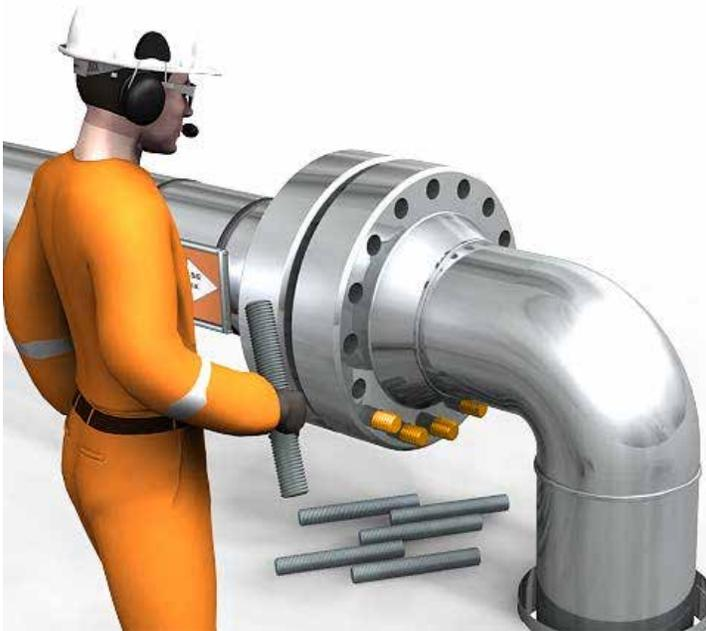
Metal rings (RTJ) shall be lubricated with a thin layer of acid-free Vaseline or thin machine oil before they are put in. This is so that point loads are avoided and so that it is easier to disassemble/remove the gasket again. Gaskets that are coated with PTFE should not be lubricated.
