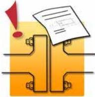
Check that the safety declaration matches the work description. Am I working on the correct flange?
