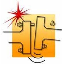
Permitted manufacturing tolerances can mean that the flange surfaces do not have the same distance around the entire flange. In other words, that the flange surfaces are not parallel. In such cases, the bolts must be tightened in the area where the distance between the flange surfaces is greatest.
