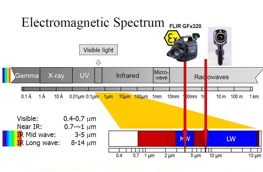
Figure 5-11 IR camera for hydrocarbons.
