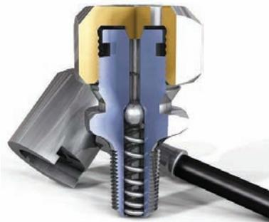
For connections with parallel threads, sealing must be achieved with a separate metal seat or sealing ring. These connections must be locked with a locking pin, or by using the lock-tight fluid specified for the installation.
