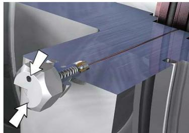
Once you are sure that the lubricating nipple is in order, screw off the cap and attach the caliper for the detergent.
