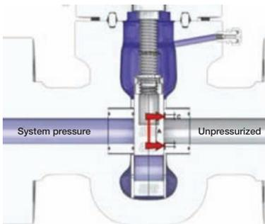
Sealing is now established on both the upstream and downstream seat – a double seal. By reducing the pressure in the valve housing, the pressure lock is removed and the valve can be opened.
