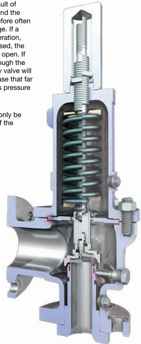
The safety valves are the last barrier against overpressure. The valves should open to a safe area for an appropriate pressure relief. They should open at a given pressure, even after not being operated over a longer period.
