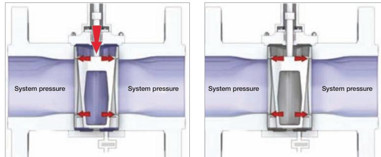
Open the drain valve to remove the pressure in the valve housing.
