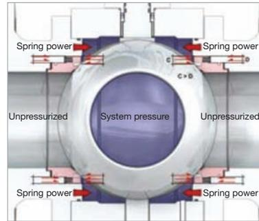
The pressure remaining in the housing, usually between 5 and 12 bar, will depend on the strength of the springs.
