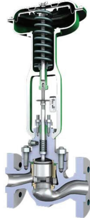
Lack of maintenance and infrequent usage can make the valve far heavier to operate. The actuator is usually designed to operate the valve under normal operating conditions. Requirements for oversizing of the actuator are common in order to increase the reliability of both the valve and the actuator.
