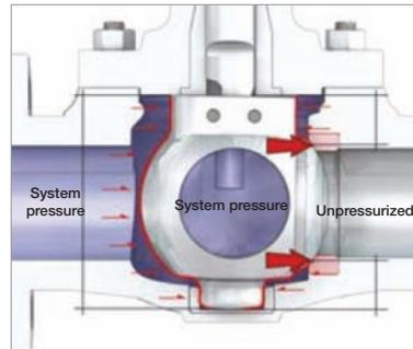
The pressure acting on the active area will increase the sealing force on the seat, since it helps to push the ball further in against the seat.
