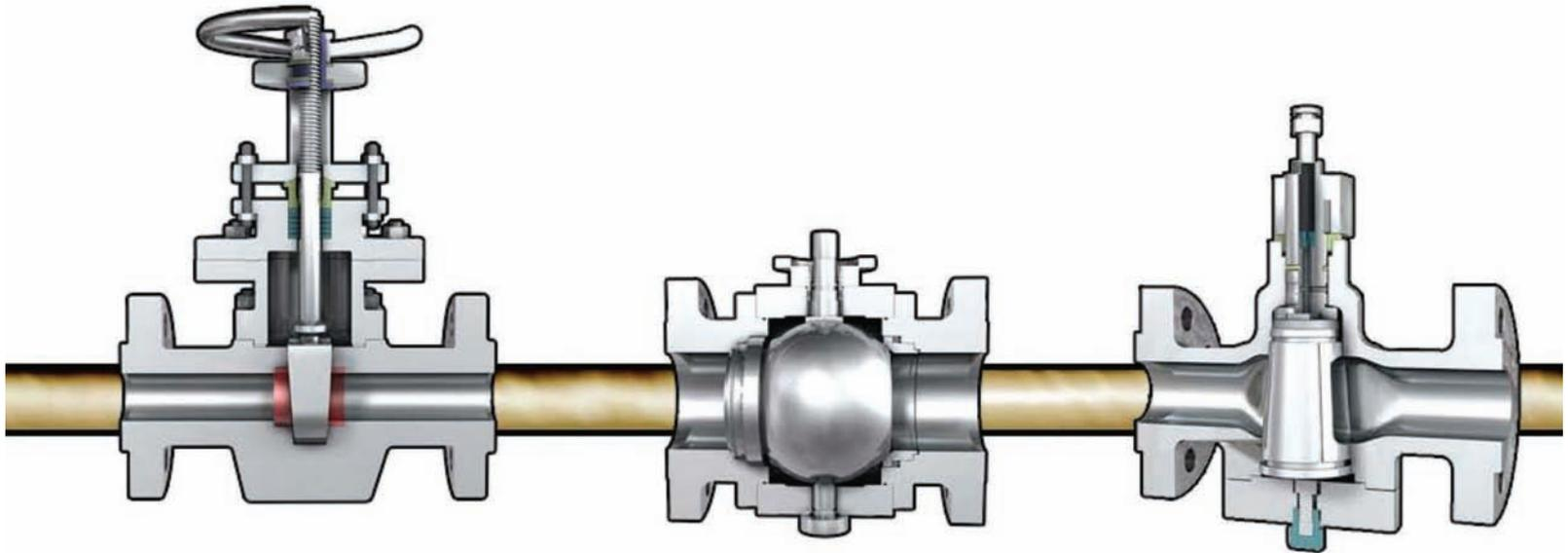
This is a line with an open wedge gate, a plug valve and a soft seated ball valve. A dirty well stream flows through a line which has been given a methanol injection to prevent hydrate formation. Important characteristics or challenges are described for each type of valve.
