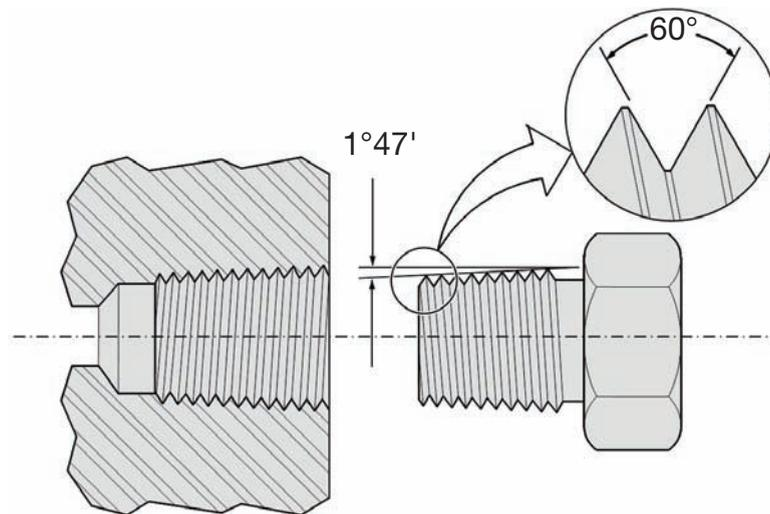
There would have to be very large deformation to achieve a continuous metal contact around the entire cross-section so that it can create a satisfactory seal. Instead, there must be a sealant that fills the gap between the threads. This could be Teflon tape or a lock-tight fluid.
