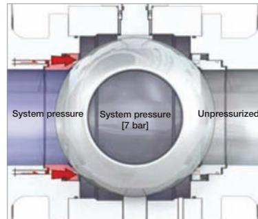
On the downstream side, it is only the spring forces that hold the seat against the ball, as it is depressurized behind the seat.
