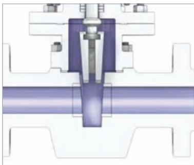
This provides a good mechanical seal with relatively little force. Although the valve seals on both seats, it is not an accepted double seal, because the valve housing cannot be depressurized.
