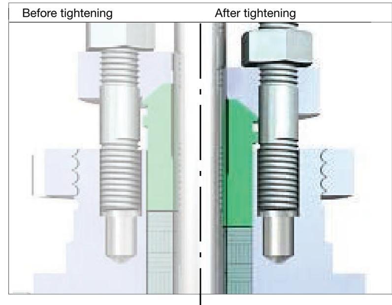
This stem seal has a seat with compressible graphite gaskets and lantern ring.
