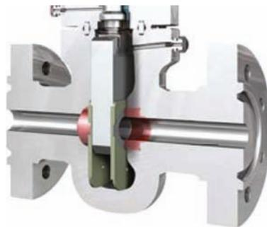
When the valve is closed, it is a good practice to turn the hand-wheel slightly towards the open position to prevent the gate locking at the bottom of the valve housing. The manufacturer's instructions should always be followed in this respect.
