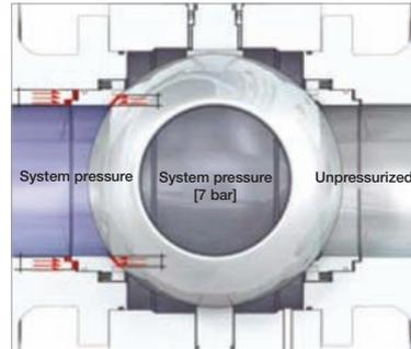
The pressure acting on this active area provides the sealing force on the upstream seat.
