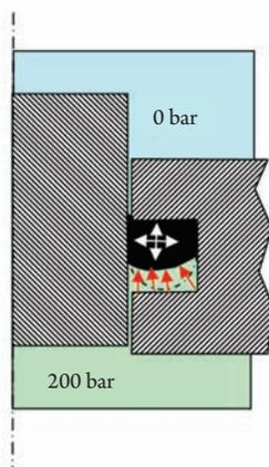
Soft seals have limited strength, so that if the pressure area is too large, the material is unable
