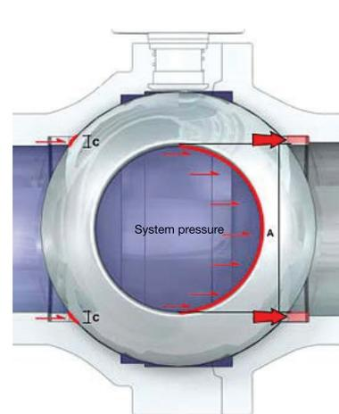
On a mounted ball valve, only the pressure forces on the seat provide sealing force. Pressure force on the ball is absorbed by the housing around the stem and therefore does not affect the seal.
