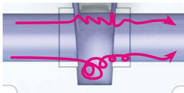
Laminar flow gives a lower pressure drop and erosion than turbulent flow. Turbulence can also break down corrosion prevention layers in low alloy or corrosion-resistant materials. With turbulence, a corrosion inhibitor has little or no effect.
