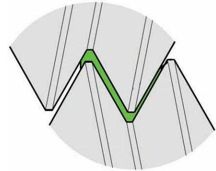
When removing plugs with tapered threads, it is difficult to control when the plug loses contact with the threads and can be shot out. The sealant will also be destroyed by unscrewing, so that it will not be possible to achieve sealing again if it is discovered that the valve seats, for example, are not tight. Therefore, plugs with tapered threads should not be unscrewed when they are pressurized. Regardless, always ensure that no person is in front of a plug when it is unscrewed.
