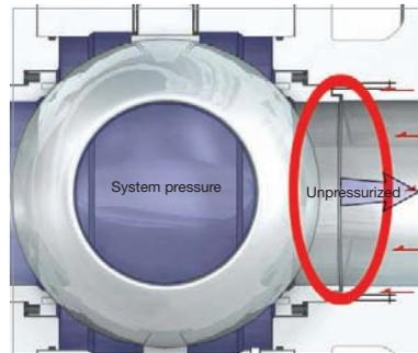
The pressure acting on this active area provides the sealing force on the downstream seat.
