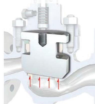
A balanced globe valve has the same pressure above and below the plug and a sealing cage, which provides only mechanical sealing force.
