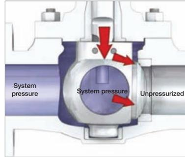
In addition, the system pressure will act with a force on the ball. Since there is pressure in the valve housing, this will press in the opposite direction on the ball.
