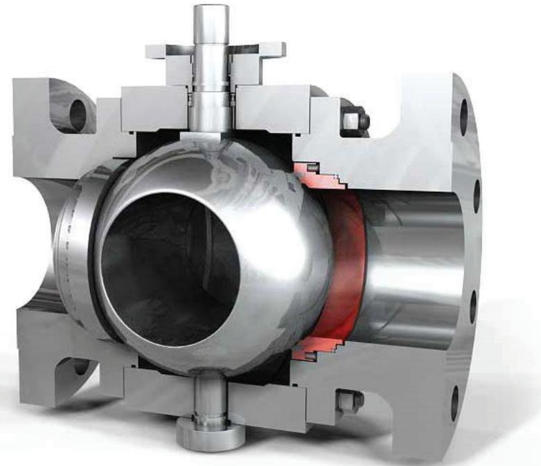
Valves with hard seats (PEEK, Devlon, etc.) should not be opened with a differential pressure exceeding 60 barg.
