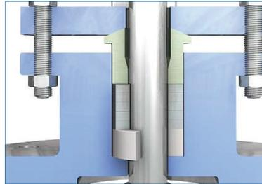
Note that for valves that have been screwed too tightly to close, the edge of the bushing under the yoke may be stretched. This may cause looseness and cause the valve knocks when it opens again. This may be an indication that the valve is in the process of being destroyed.
