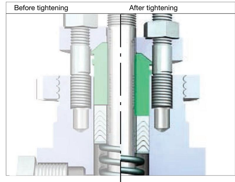
This stem seal has a coil spring between the lower scraper ring and the seat with PTFE V-gaskets.
