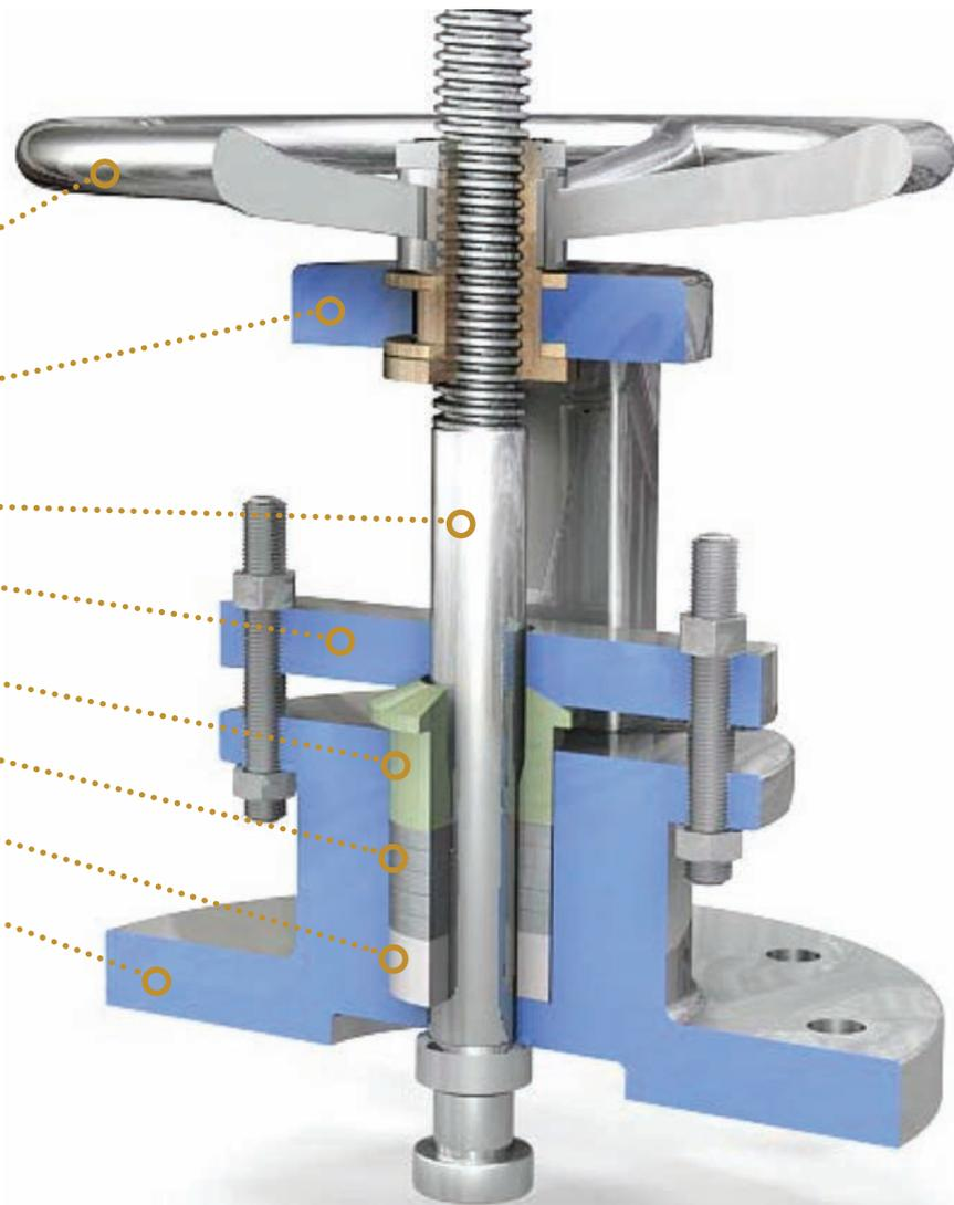
Troubleshooting in connection with valve tops as shown in the figure, is usually performed in connection with stem leaks or operational problems.
