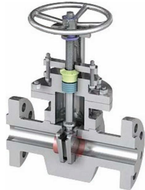
A valve should always be closed by turning clockwise. On normally operated valves, the stem will go down to close. If the valve is reverse operated, the stem will go up to close.
