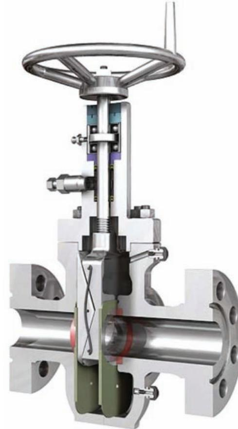
**!** This valve must be tightly screwed in the closed position so that the gate will expand against the seats. In the open position, the valve must also be screwed tightly. This is because the gate must expand against the seats.
