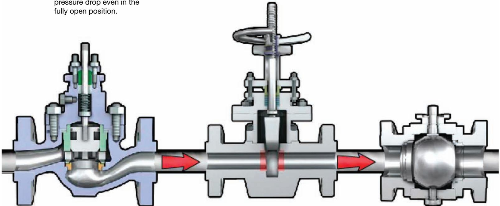
This is a line with an open wedge gate, a control valve and a soft seated ball valve. Gas passes through the line at high speed. Important characteristics or challenges are described for each type of valve.
