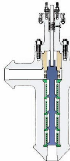
There are a number of trims especially designed to control the pressure drop across the valve so that it does not fall below vaporization pressure.
