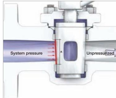
This force pushes the plug towards the downstream side and toward the Teflon sleeve so that the valve seals.
