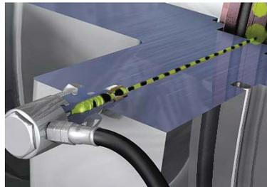
Pump in some kind of detergent from the hand pump. The detergent dissolves the deposits and friction between the seat and the seat pocket is reduced.
