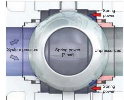
Since the downstream negative area is greater than the downstream positive area, the seat will release when the pressure in the housing exceeds the spring force.
