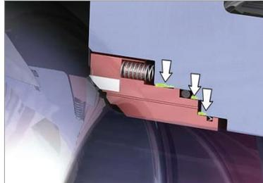
In the closed position, the deposits now come into contact with the seat's soft seals at the indicated points. At exactly these points, the soft seal will climb up on the deposits so that the seat no longer comes properly into contact with the ball. The valve will leak.
