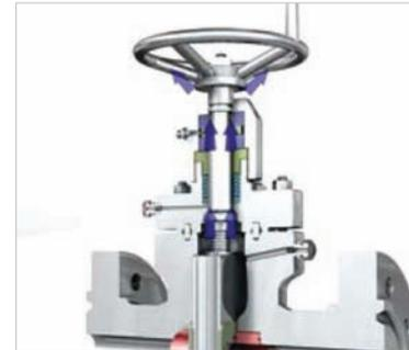
The first thing to do is to loosen the stem cup under the wheel. The stem is now pushed into the backseat position by the system pressure in the valve housing.
