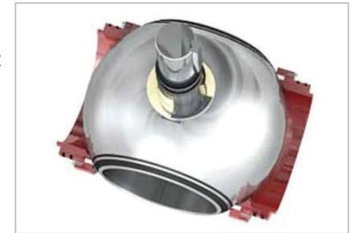
Remove deposits on the ball by rotating it 5-10 degrees back and forth 4-5 times in both the open and closed position. This applies in cases where there is both one and two lubricating nipples into each seat.
