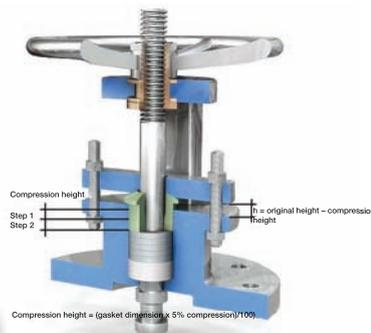
Note! Make sure the pressure gland is horizontal and does not scrape against the stem during compression.
