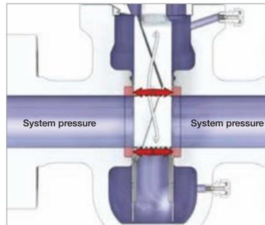
In order to create a seal between the housing and the barrel, both gate halves must have additional sealing surface, as shown in the figure. Valves without such additional sealing surfaces on the gate halves, will not have this sealing function.
