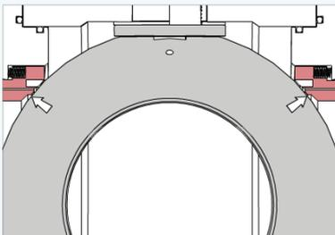
If the pressure upstream is now reduced, none of the seats are in contact with the ball and the valve will leak when the system is pressurized.
