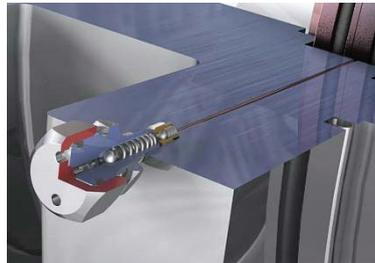
The holes in the cap can now be used to check for leaks, as the extra seal in the cap has gone.
