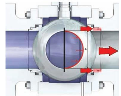
*The figure shows the pressure forces in a ball valve with floating ball.*
