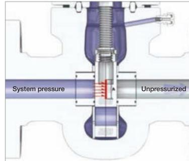
Because of the seat's design, the pressure in the valve housing will also act on area C, which provides additional sealing force on the downstream seat.
