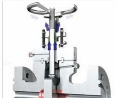
A rising stem must be set in the upper position to go in backseat. Check the seal by placing a stinger on the lubricating nipple.
