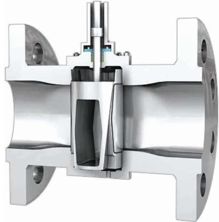
When the valve is closed, the slips are pushed against the housing on both sides, and there will be a locked-in pressure in the housing.
