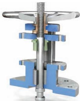
3) Use a gasket blower to remove the old stuffing box. Observe safety precautions during use. Personal protective equipment is required.
