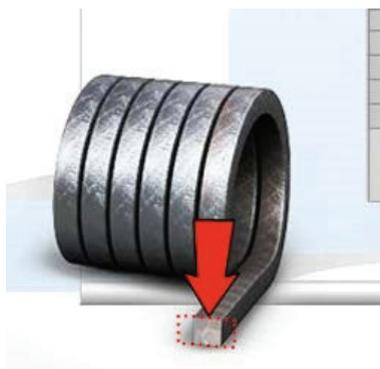
8) Adjust the carbon sleeve measurement to fill the extra distance beyond five rings.
