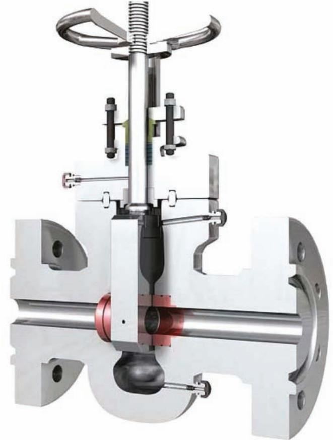
When the valve is closed, it is a good practice to turn the hand-wheel slightly towards the open position to prevent the gate locking at the bottom of the valve housing. The manufacturer's instructions should always be followed in this respect.
