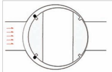
The system pressure acts on the plug over area A and provides a force equal to the system pressure multiplied by the area.
