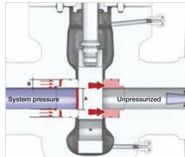
For the upstream seat, the sealing force will be provided by the system pressure acting behind the upstream seat, area B.
