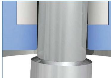
When the valve is operated, vertical scratches may occur on the stem. It is important that the stem is always in the backseat when the pressure gland is tightened. Rising non-rotating stem – vertical scratches. Ascending rotating stem – spiral stripes.
