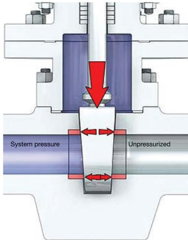
A solid gate valve with fixed seats has pressure forces that are absorbed by the downstream seat.
