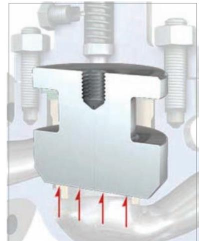
There are two main types of stem seals for control valves – with and without spring load. When the valves arrive from the manufacturer, it is usually without a tightened stuffing box. Therefore, tightening should usually be performed before the valve is put into operation. The procedures for installing and tightening the stuffing box vary and are specially adapted to the materials, construction and pressure ratings.
