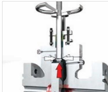
When the backseat seal has been checked, replacement of the stem gaskets can be carried out.
