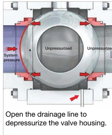
The differential pressure between the upstream and downstream side establishes a double seal by the ball being pressed against the downstream seat and the upstream seat is pushed against the ball.
