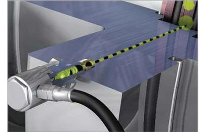
When pumping in lubricant, the friction that prevents movement of the seat will be reduced.
