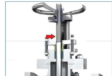
The usual procedure is that it is replaced with original sealing according to the parts list or sealing of type low density braided 1% reinforced and 99% pure graphite.
