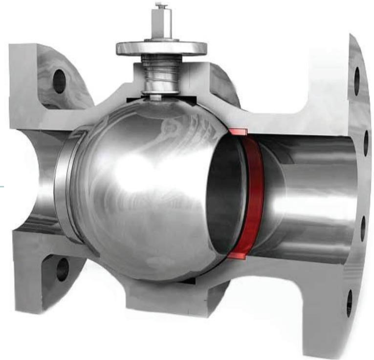
Conventional valve with soft seats should usually not be opened with a differential pressure exceeding 20 barg.
