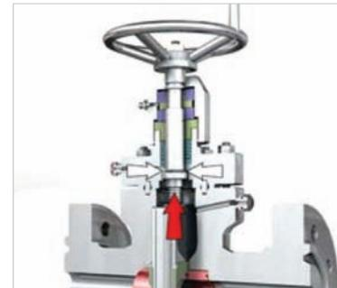
Check the seal by placing a stinger on the lubricating nipple. When the backseat seal has been checked, replacement of the stem gaskets can be carried out.
