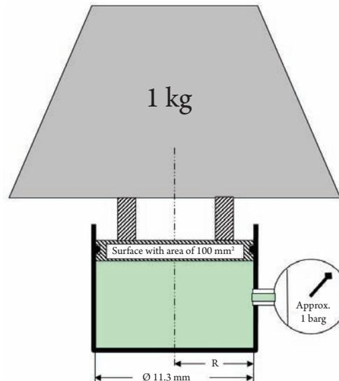
The area of a circular surface is calculated by the radius squared, multiplied by Pi ( $\Pi = 3.14$ ).
