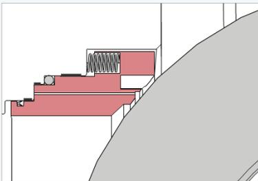
As can be seen, the upstream seat does not move – it remains in the seat pocket.
