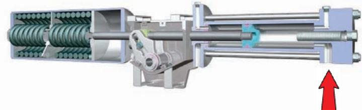
On certain valves that are critical for safety, there is a backup system to ensure that the valve can be opened and closed a certain number of times. For safety-critical maintenance operations, the hydraulic system, including the backup system, must be disconnected and have a drainage point against the actuator. This is done to prevent pressure buildup in the hydraulic system that could cause undesired valve operation.
