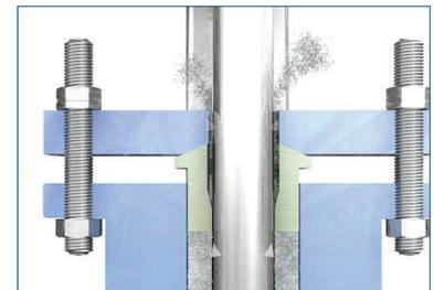
Note! This can only happen with the molded type (Grafoil), not with the reinforced braided.
