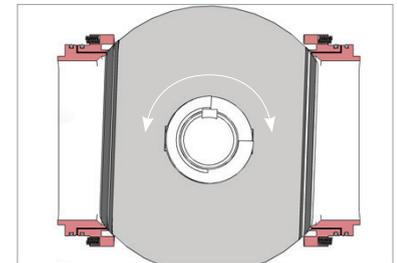
When the ball is operated in this way, the seats will work like scraper rings, and the dissolved deposits will disappear.
