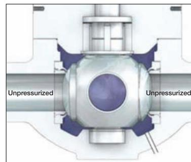
The pressure will press the ball against the seats, but there is no danger of pressure lock, since the seats are fixed and the ball will move from the seats on both sides when the valve is opened. When the valve starts to open, it will be slightly heavier to operate.
