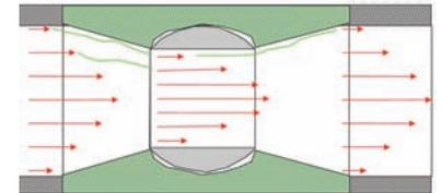
of equipment or elbows that generate turbulence, this can create conditions that alter the characteristics of the valve. For example, a wedge-gate valve will be able to operate satisfactorily with moderate velocities if the flow upstream is laminar.
