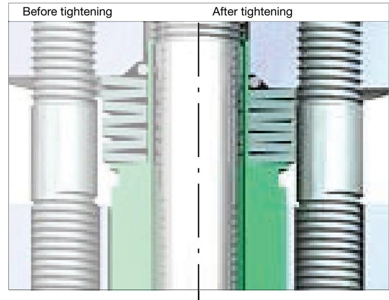
The stuffing box shown here consists of V-gaskets with a lantern ring between and a spring assembly above the pressing ring.
