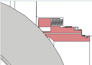
When the downstream pressure decreases, the differential pressure over the ball could deform the ball and trunnion so that the downstream seat is pressed into the seat pocket.
