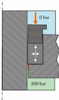
Although the gland force acts parallel to the gap to be sealed, this force will produce pressure in the graphite so that a sealing force is created normally on the stem and valve housing. The size of this force in relation to the gland force depends on the consistency
