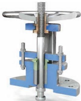
2) Remove the gland nuts. Lift up the pressure gland and the pressure sleeve and bind them securely.
