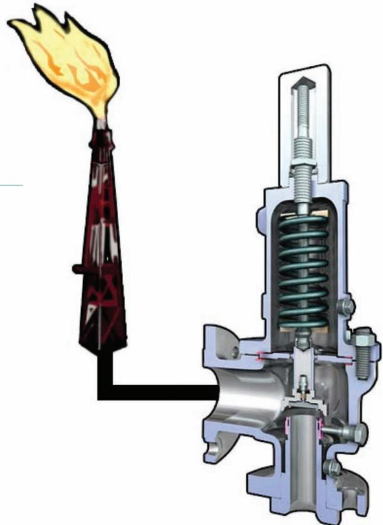
When the pressure on the disk's area produces an opening force that exceeds the spring pressure, the valve will open. When the valve has opened, the spring is compressed.
