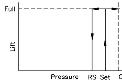
A pilot that is modulating, bleeds off the desired pressure above the piston to provide an opening adapted to the pressure increase in the system.
