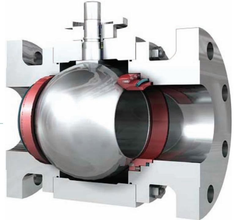
! The valve seats can be tested by reducing the pressure in the valve housing. Conventional valve with soft seats should usually not be opened with a differential pressure exceeding 20 barg.
