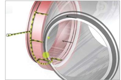
When there is only one lubricating nipple on each seat, it will not be possible to wash off the valve seat for more than one side of the seat.
