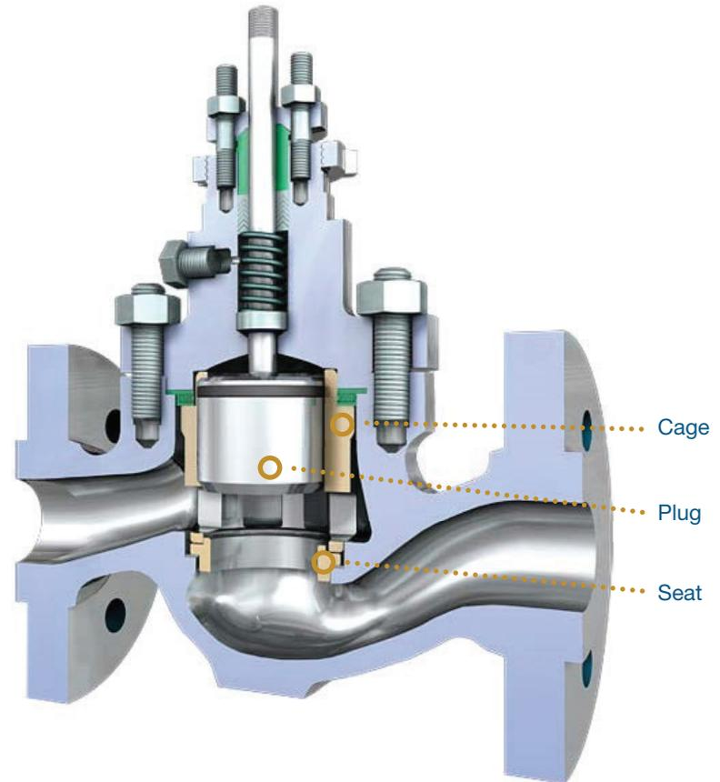
⚠ To reduce the risk of cavitation, cage guided valves should not have less than 20% real opening, including the dead band.
