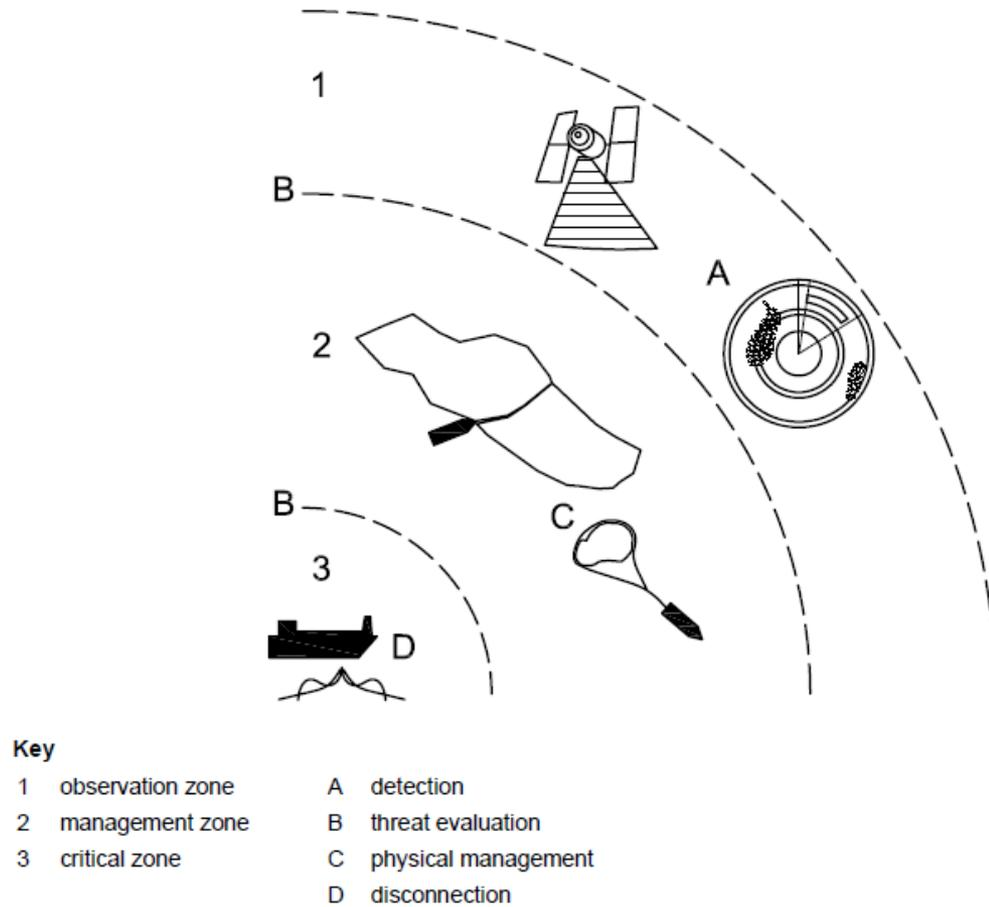
Figure A.17-1 — Typical components of an ice management system
