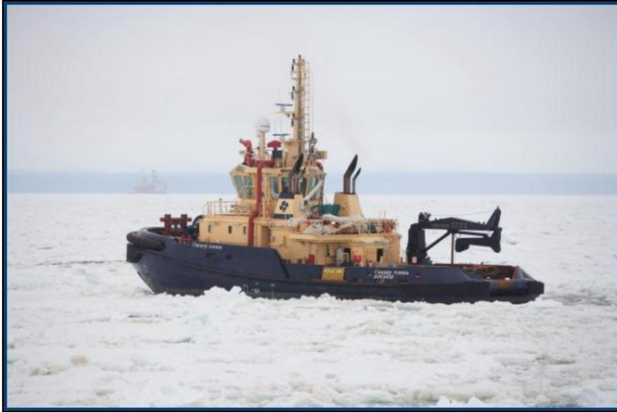
Operations in Prigorodnoye require support of the harbour tugs. Sakhalin Energy operates four purpose built ice class 1A tugs equipped with Aquamaster propulsion system (Z drive).
