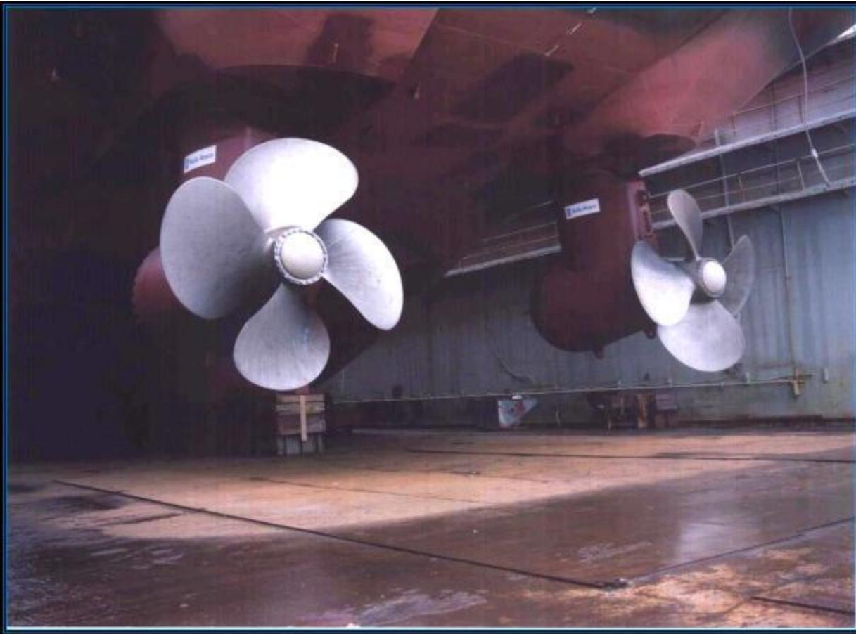
The Aquamaster propulsion systems installed on the vessels are of two types:
