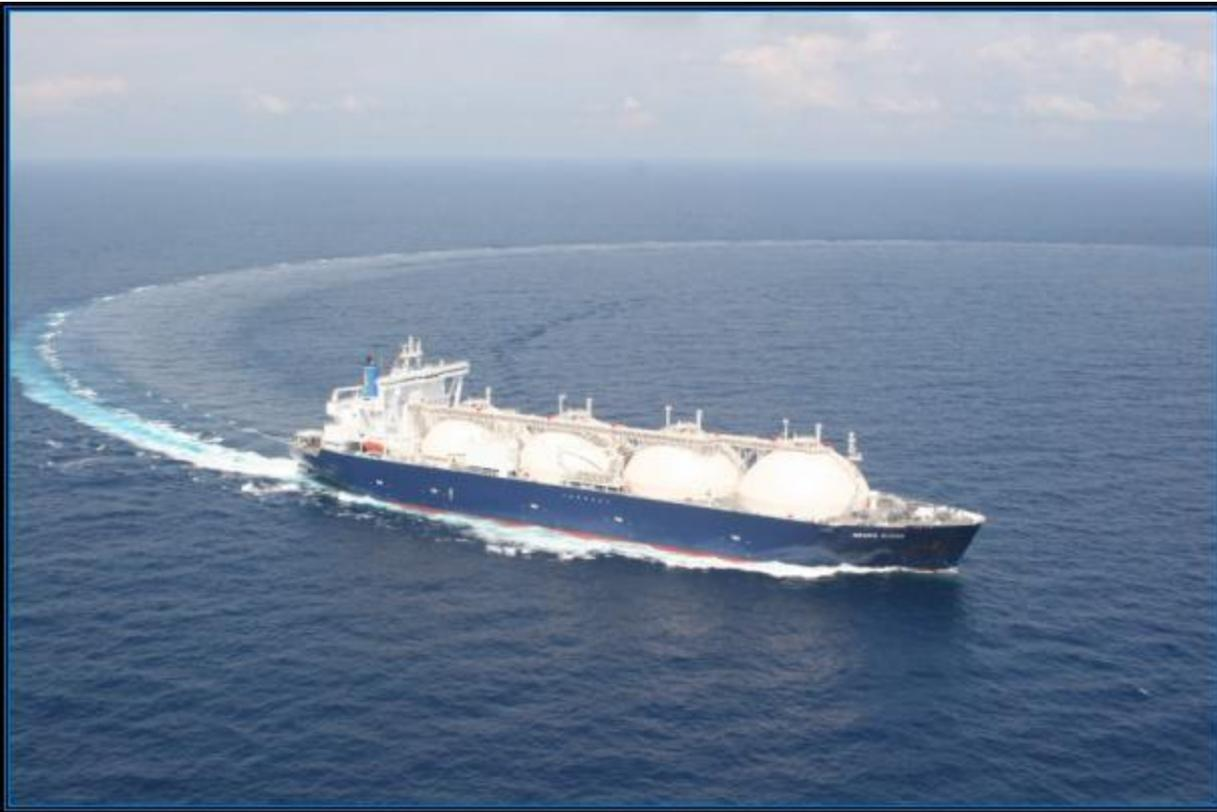
The 145 000 m<sup>3</sup> LNG carrier Grand Elena shown here is an Ice Class 1C vessel purpose built for the project. It is one of 5 purpose built vessels for the project.
