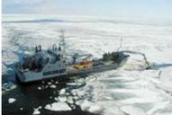
Multipurpose <b>response vessel for ice concentrations up to 30%</b> . | Response measure IceRV equals a multipurpose vessel system equipped for combating oil in the marginal ice zone. The system is primarily set up for operations in ice up to 30 % concentration and comprises of kits for 1) mechanical recovery, 2) ISB and 3) dispersant application in ice. <b>NOTE: this response measure has not been modelled but assessed quantitatively in a calculator tool.</b> |
