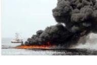
Open water <b>in-situ burning</b> system                               | Response measure ISB equals a future response concept for In Situ Burning in open waters. The measure is based on a modern OR stand-by or supply vessel with oil detection capacities (IR and oil radar) and carries an additional ISB kit with fire booms and a surface ignition system. Towing vessels could be daughter crafts or fishing vessels.                                                   |
