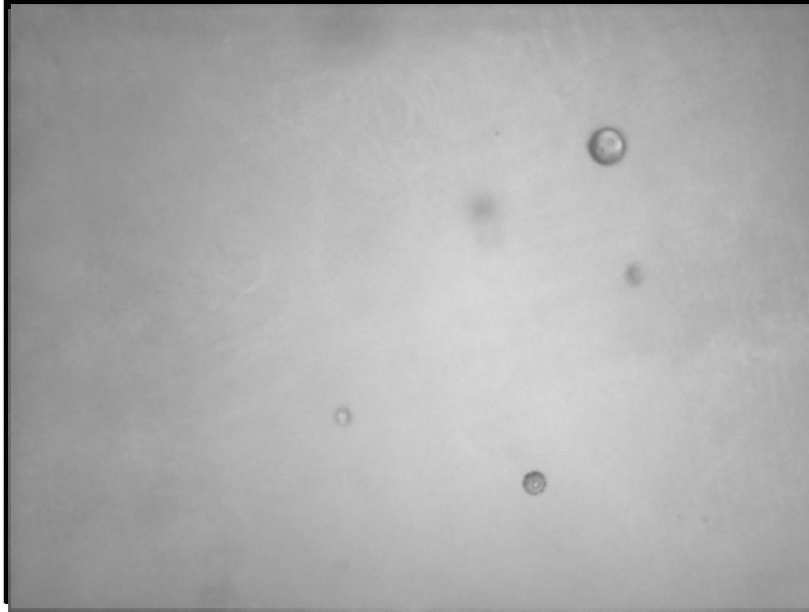
A stream of raw images (400 – 4500) from each Tower Basin experiment is processed by an automatic droplet analysis system
