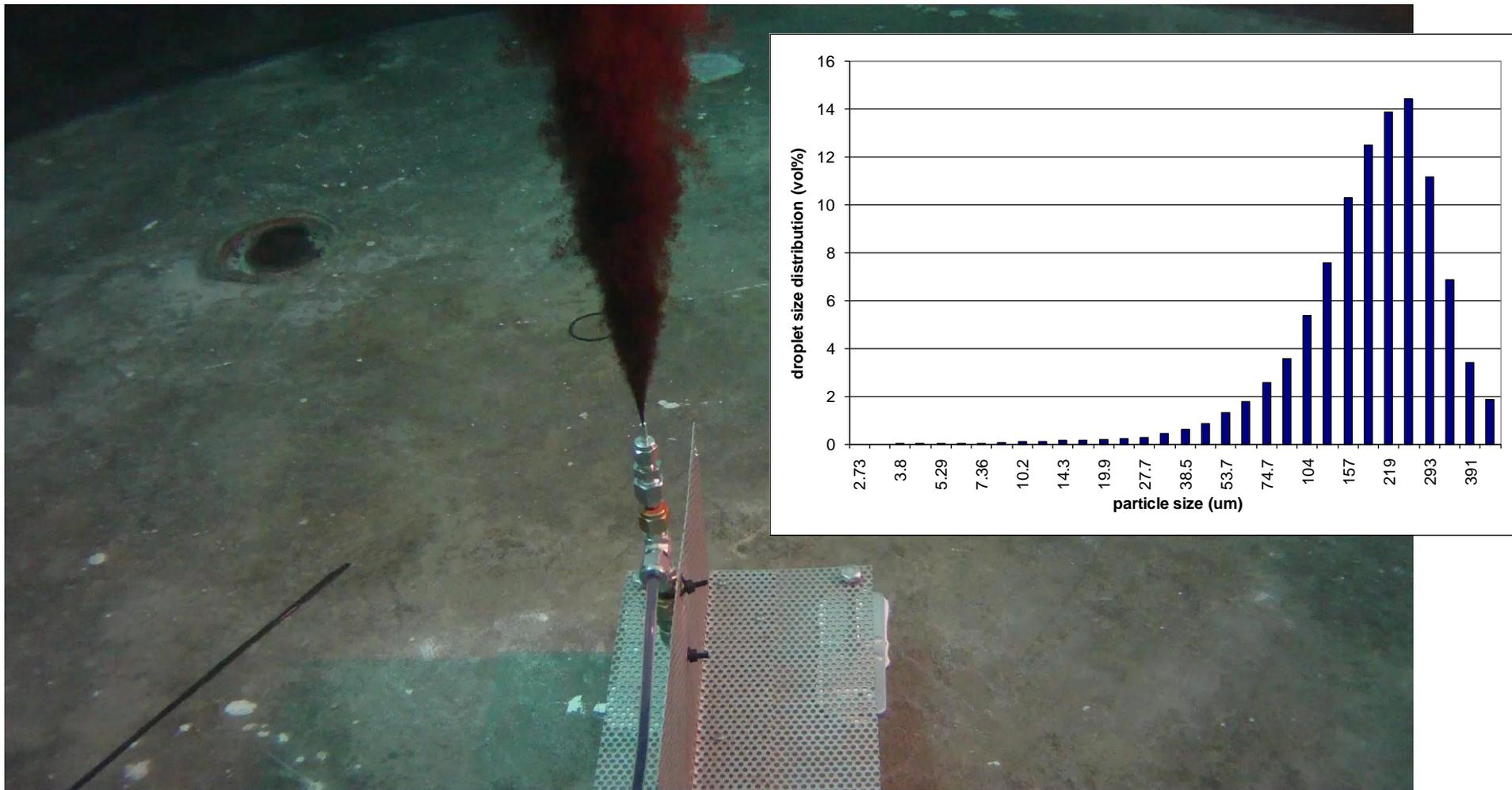
Release of Oseberg oil: Diameter 1.5 mm, rate: 1 L/min (3 x 90 sec)
