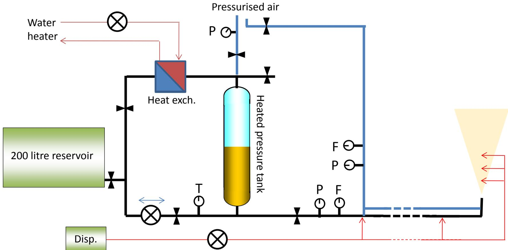
Principle overview of the set-up showing how oil, gas (air) and dispersant will be released during the experiments.
