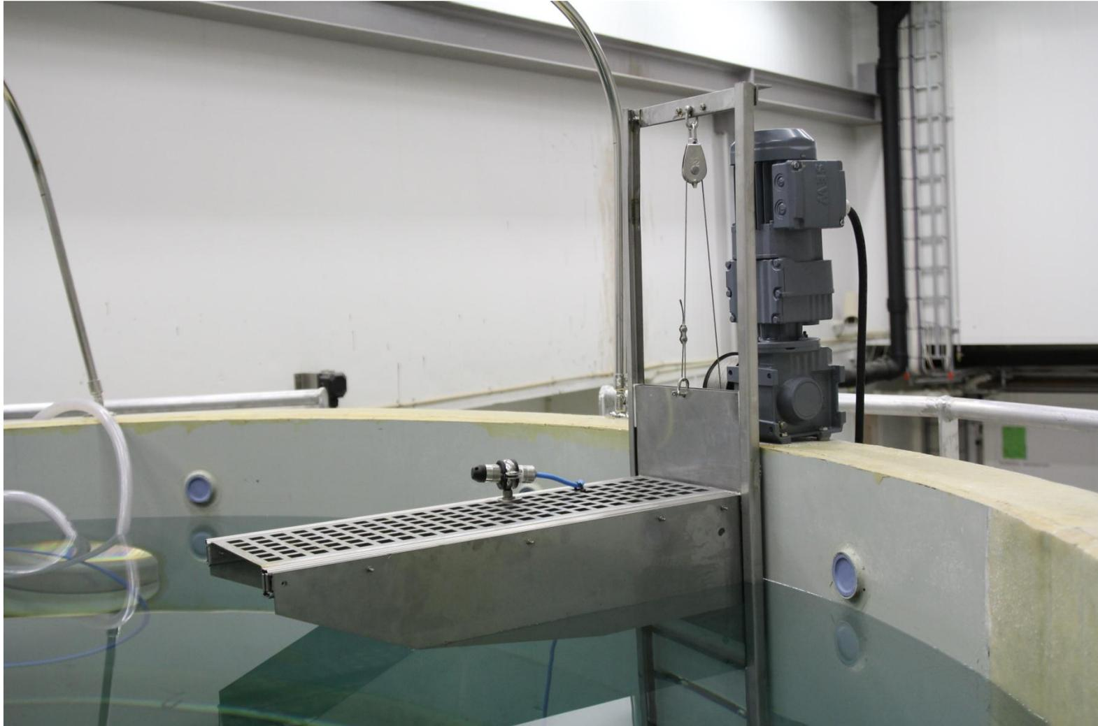
Remotely operated (vertical/axial) instrument platform, with depth sensor (1-6 m)
