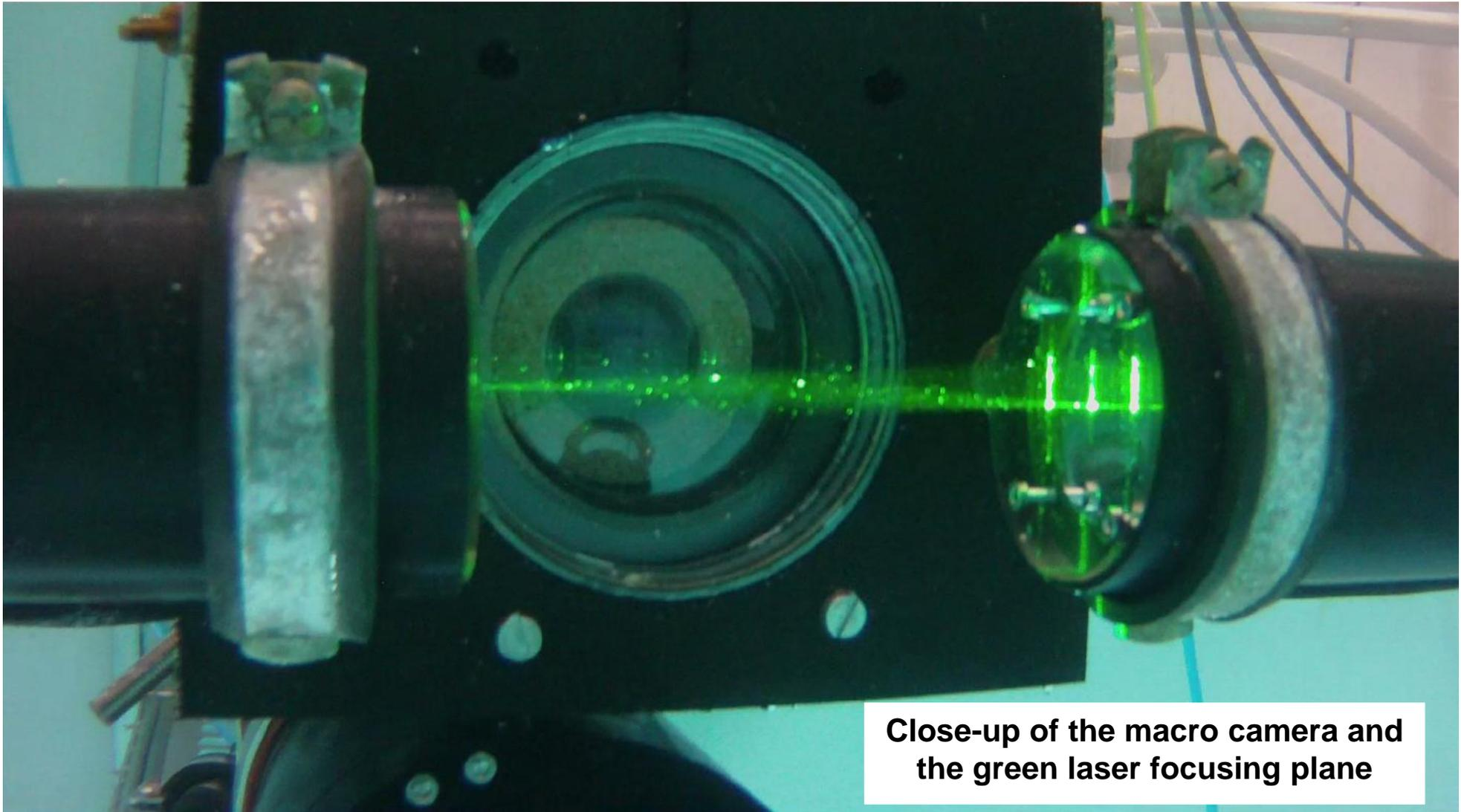
Close-up of the macro camera and the green laser focusing plane
