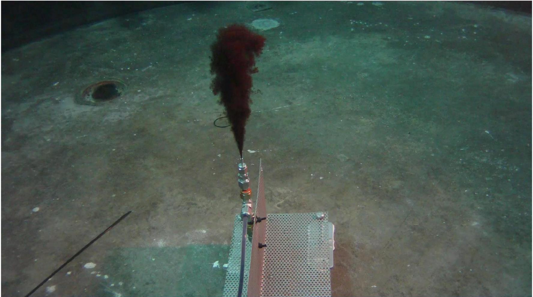
Release of Oseberg oil: Diameter 1.5 mm, rate: 1 L/min (3 x 90 sec)
