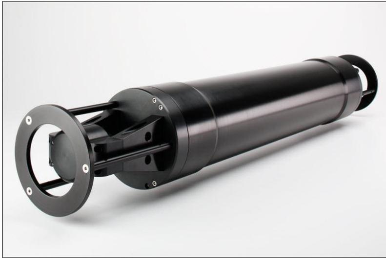
Detecting particle size distribution by laser diffraction technique.
