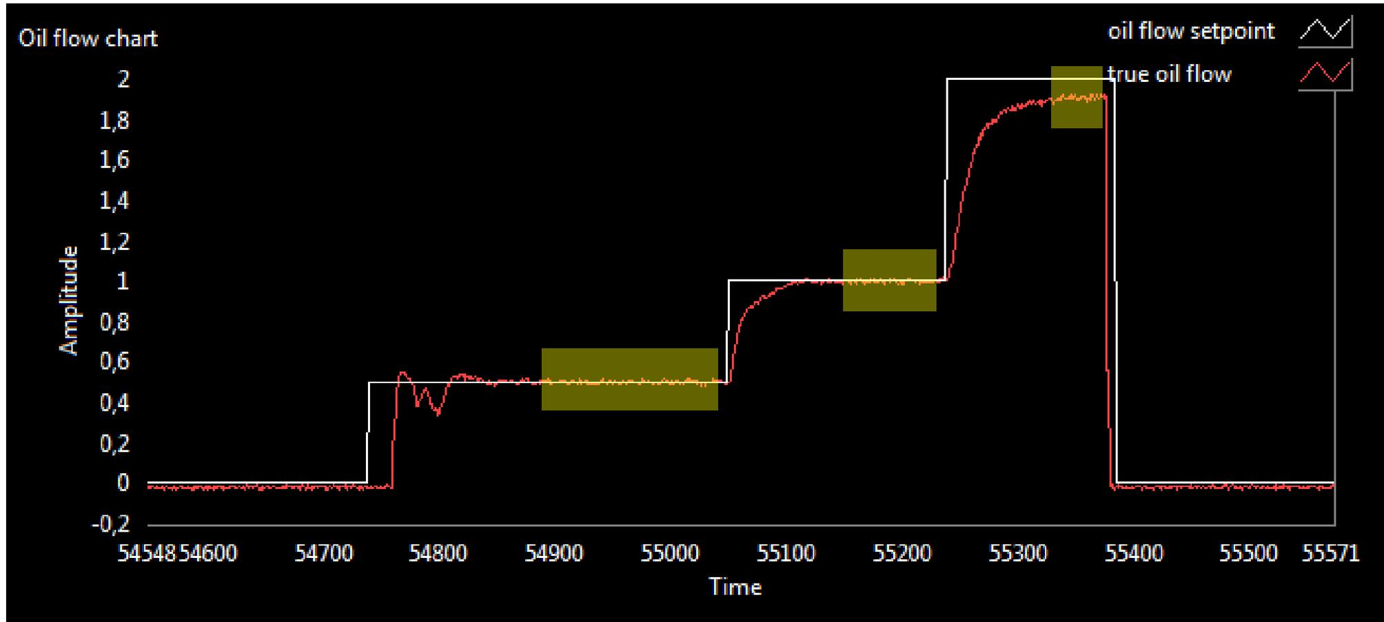
Control and monitoring of oil flowrates for a typical experiment (one nozzle three flow rates)
