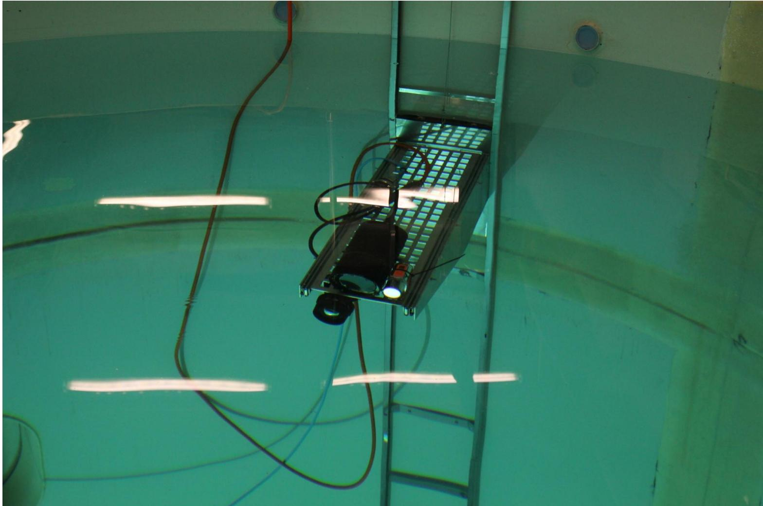
Cameras (zoom and fixed) and light mounted on instrument platform
