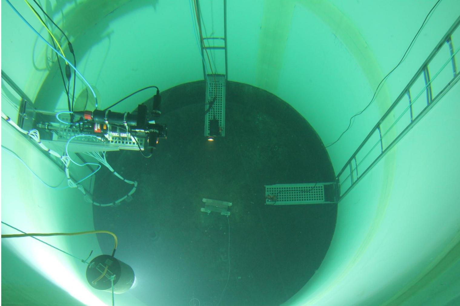
Droplet size monitoring equipment at 3 meters dept, cameras at bottom
