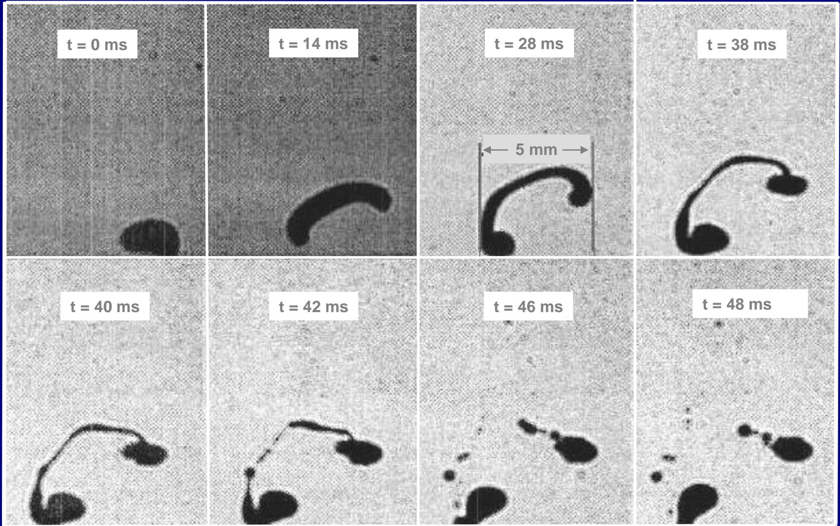
Extracted images from cinematic digital holography of turbulent break-up of crude oil mixed with dispersants into microdroplets
