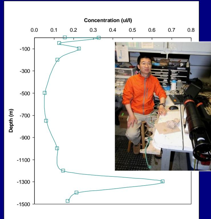
Small particles (2.5 - 60µm) were indicative of oil droplets in the subsurface plume
