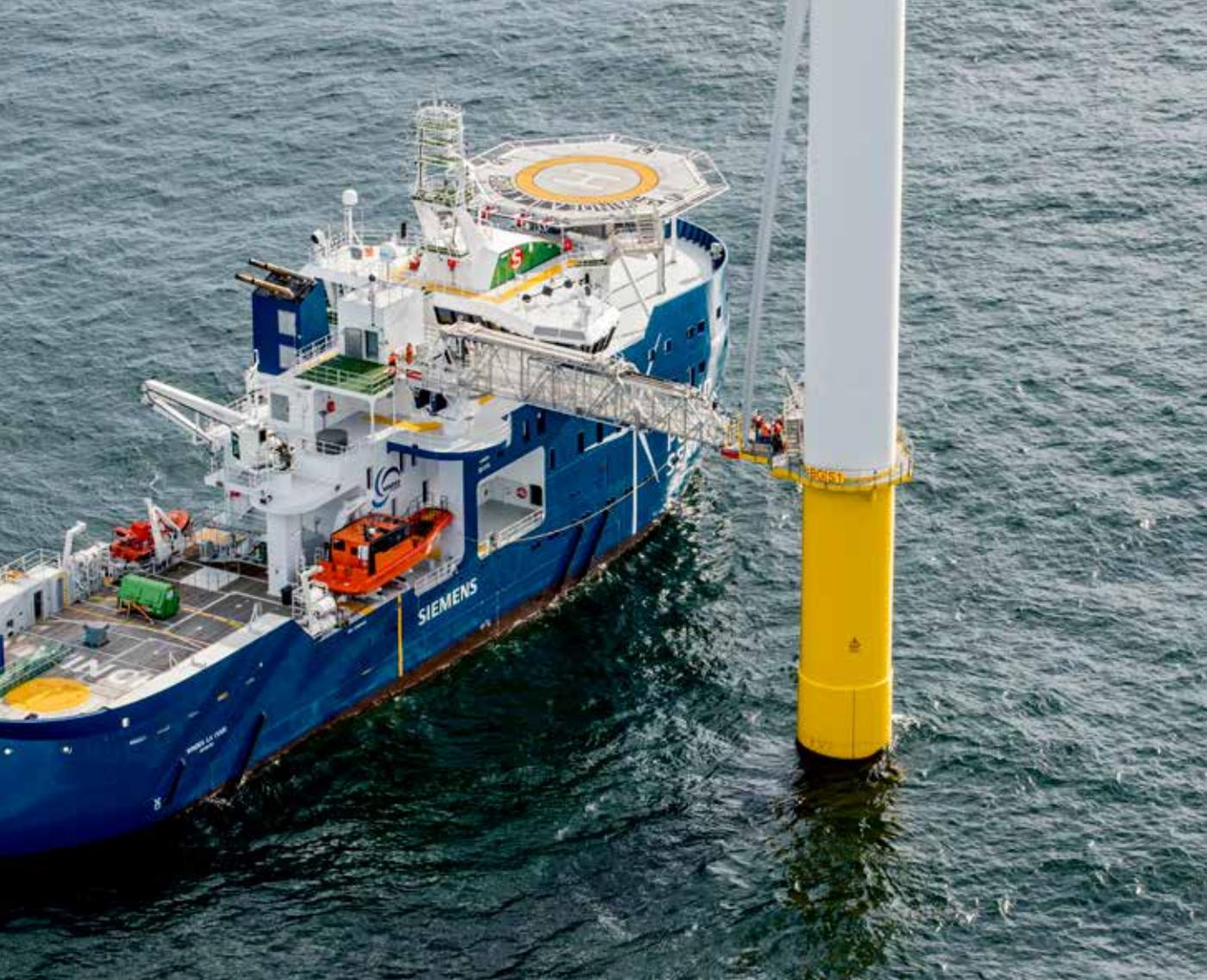
lift in an adjustable pedestal and across the gangway on electric trollies. That means technical personnel do not have to carry tools and equipment. Work on and maintenance of the turbines can be carried out without the need for cranes.
